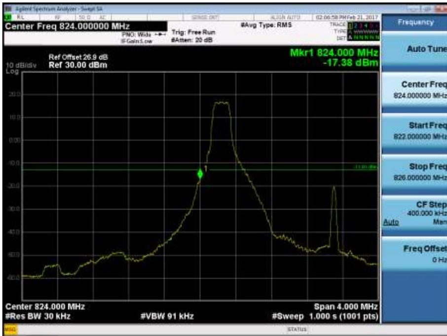
BAND 5. Lower Band Edge Plot (3M BW Ch.20415 QPSK\_RB15\_Offset 0)
