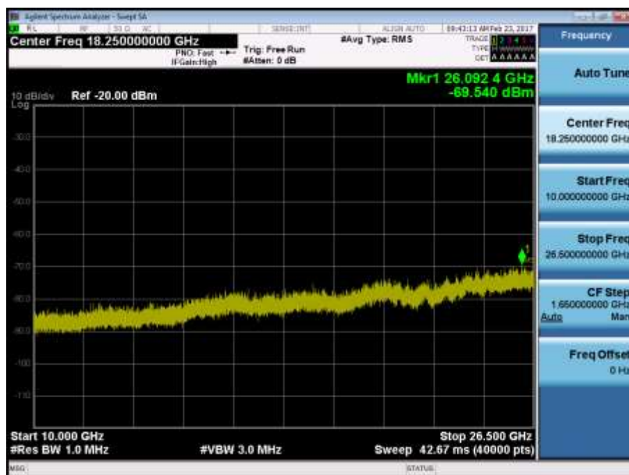
BAND7. Conducted Spurious Plot 2 (20MHz Ch.21100 QPSK RB 1, Offset 0)
