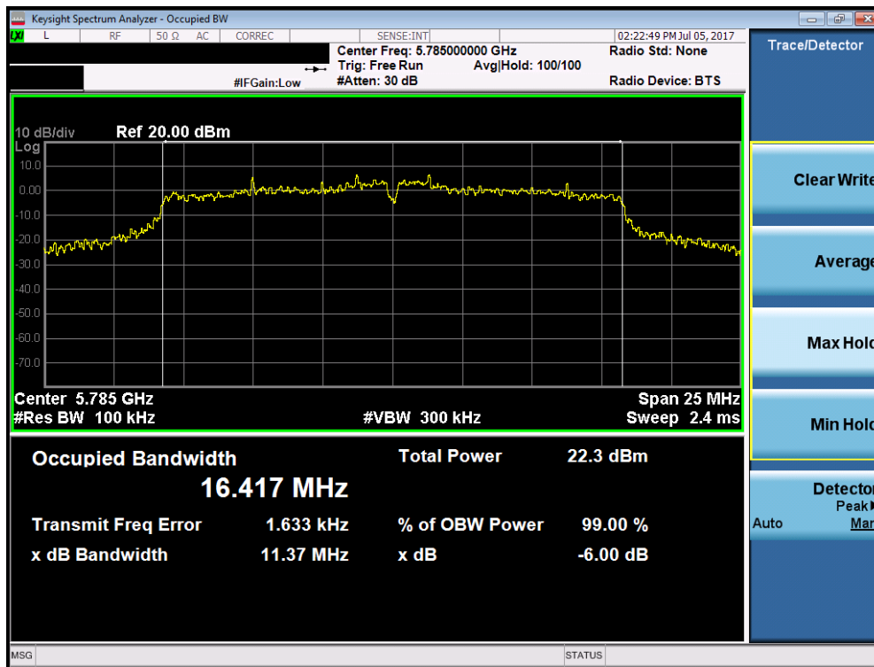
Plot 7-60. 6dB Bandwidth Plot (802.11a (UNII Band 3) – Ch. 157)
