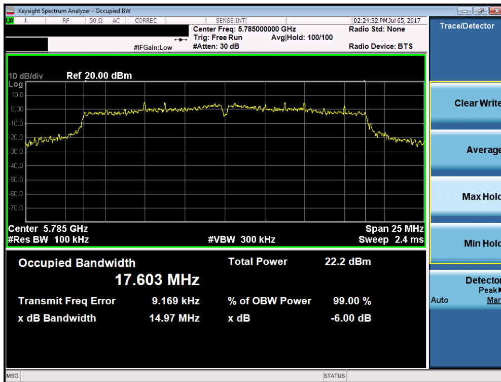
Plot 7-63. 6dB Bandwidth Plot (20MHz BW 802.11n (UNII Band 3) – Ch. 157)
