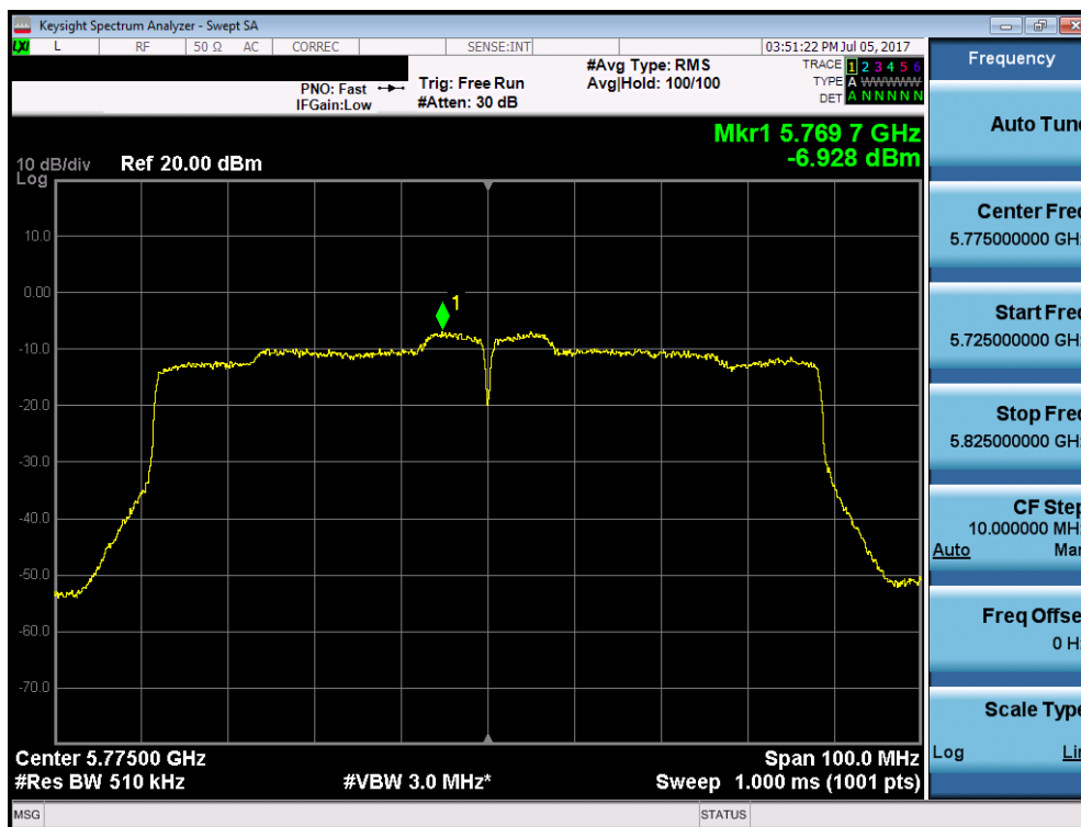
Plot 7-114. Power Spectral Density Plot (80MHz BW 802.11ac (UNII Band 3) – Ch. 155)
