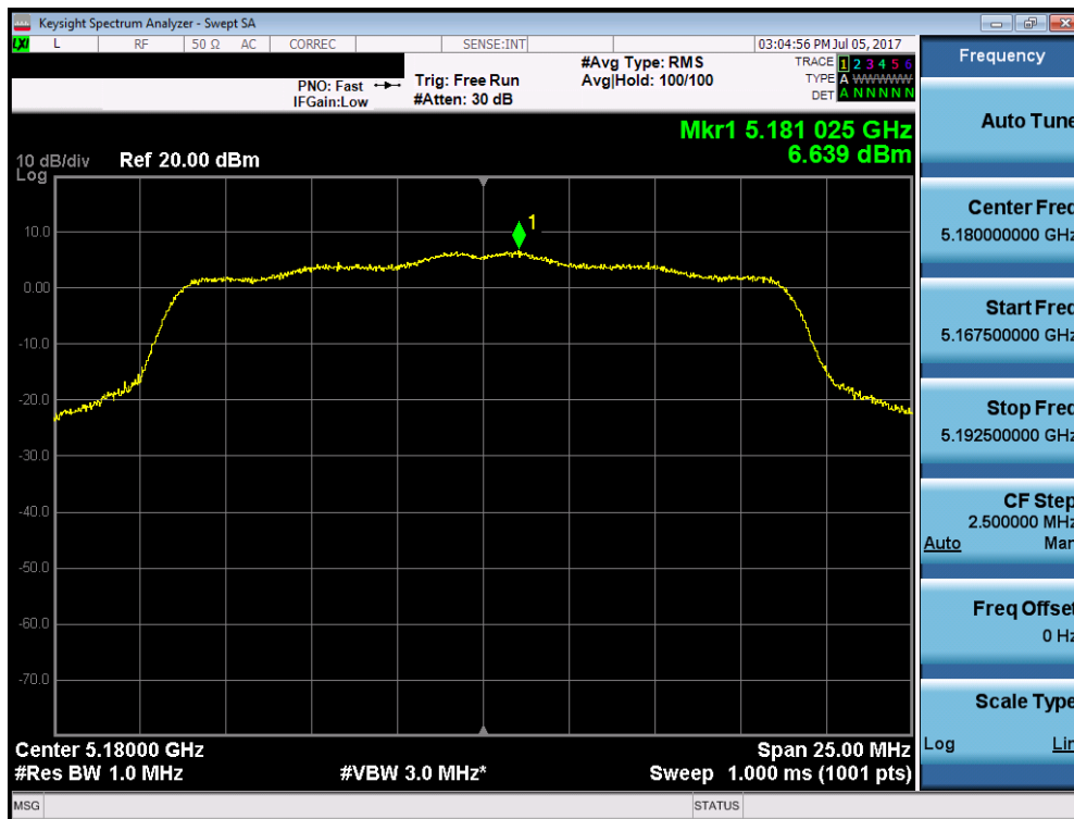
Plot 7-80. Power Spectral Density Plot (20MHz BW 802.11n (UNII Band 1) – Ch. 36)
