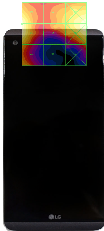
Figure 17-4 E-Field WD Scan overlay
