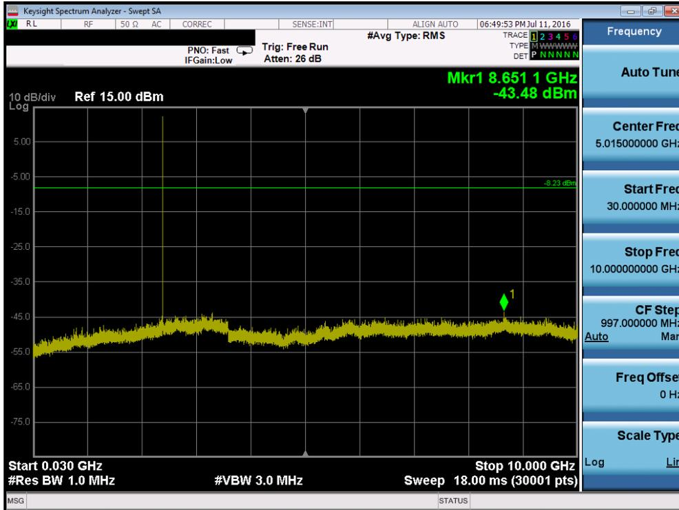
Plot 7-36. Conducted Spurious Plot (Bluetooth, 1Mbps – Ch. 0)
