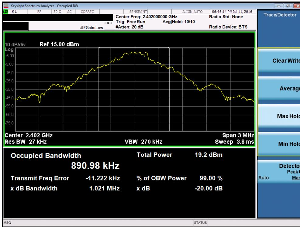
**Plot 7-1. 20dB Bandwidth Plot (Bluetooth, 1Mbps – Ch. 0)**
