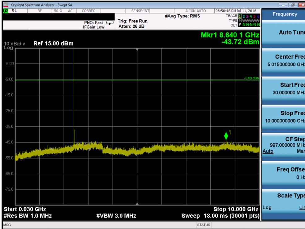
Plot 7-38. Conducted Spurious Plot (Bluetooth, 1Mbps – Ch. 39)
