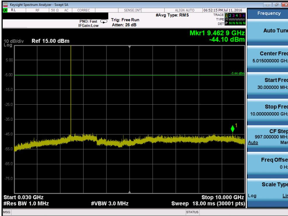
Plot 7-40. Conducted Spurious Plot (Bluetooth, 1Mbps – Ch. 78)
