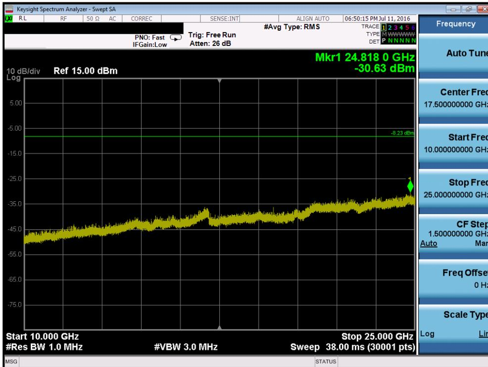
Plot 7-37. Conducted Spurious Plot (Bluetooth, 1Mbps – Ch. 0)
