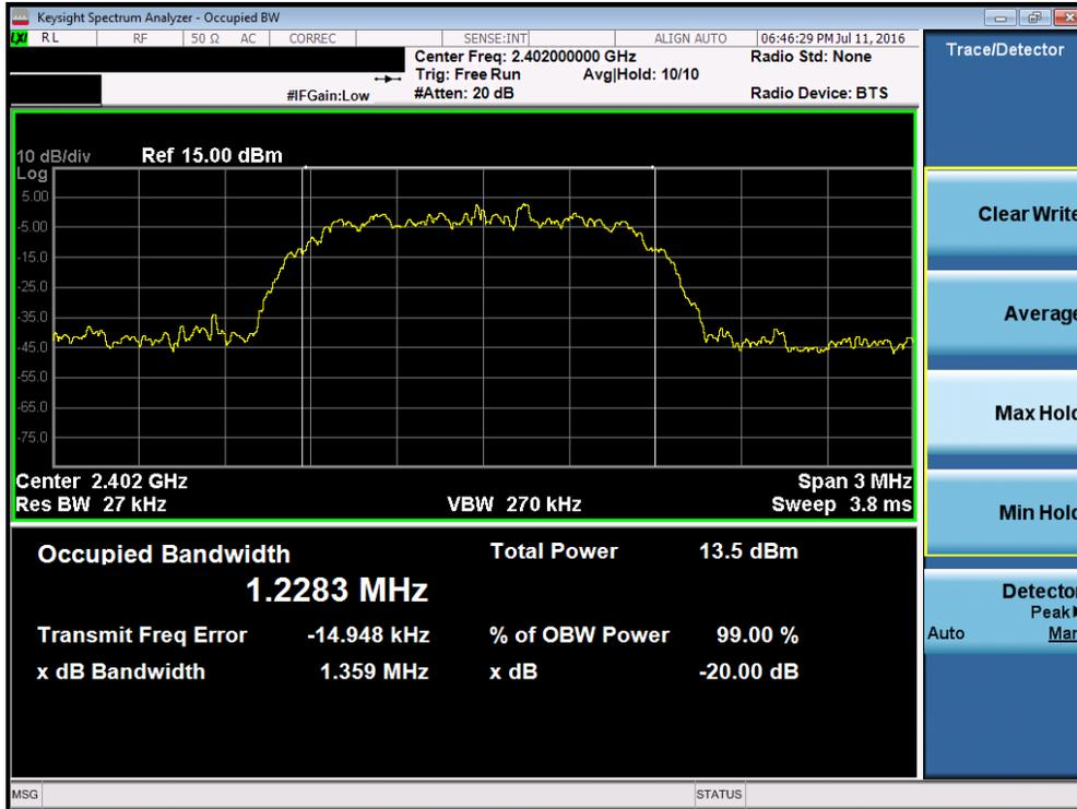
Plot 7-4. 20dB Bandwidth Plot (Bluetooth, 2Mbps – Ch. 0)
