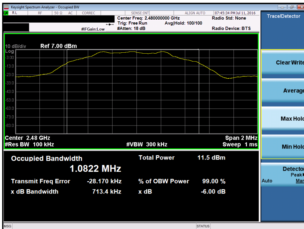
Plot 7-3. 6dB Bandwidth Plot (Bluetooth (LE) – Ch. 39)
