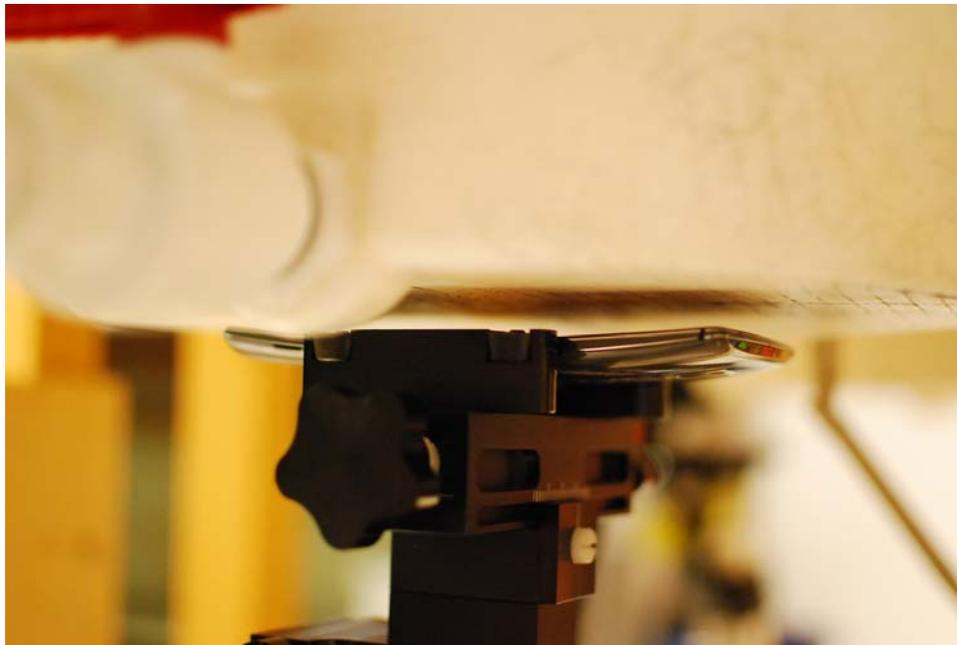
**SAR Test Setup Photo 6: Front at 0.8 cm**
