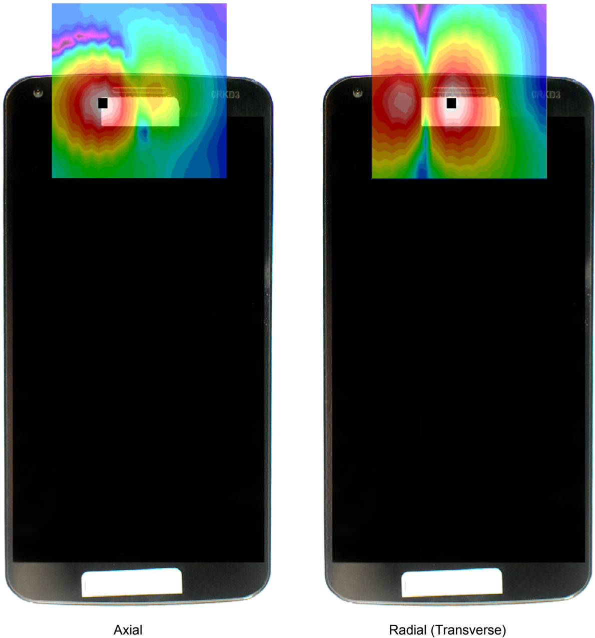
Figure 13-3 T-Coil Scan Overlay Magnetic Field Distributions
