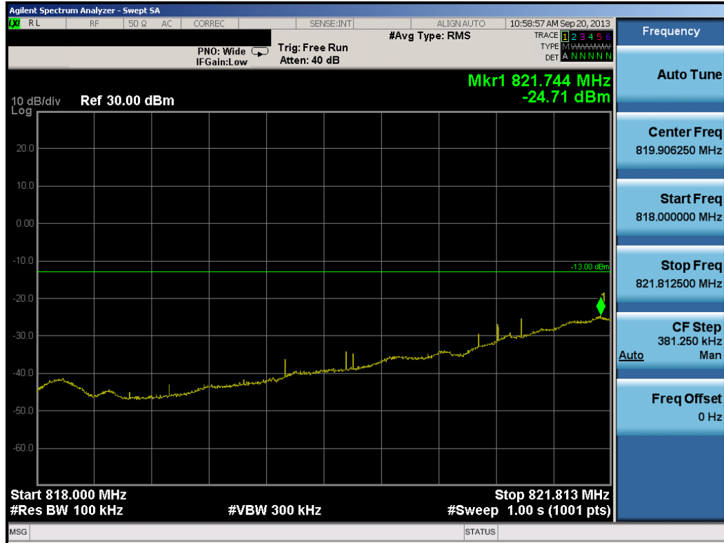
Plot 7-9. Lower Extended Band Edge Plot (Ch. 670)
