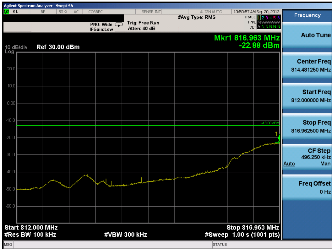
Plot 7-4. Lower Extended Band Edge Plot (Ch. 476)
