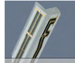
Figure 5-1 E-field Free-space Probe
