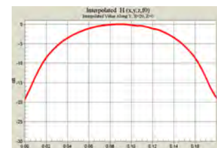
Figure 7-5 2-D Interpolated points from scan along dipole axis
