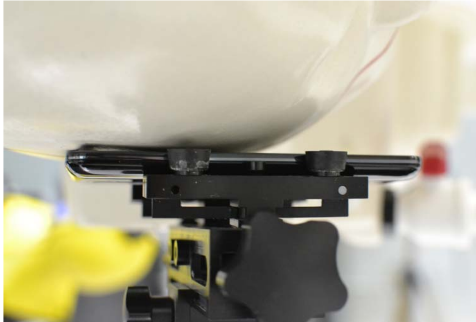
SAR Test Setup Photo 1: Right Cheek
