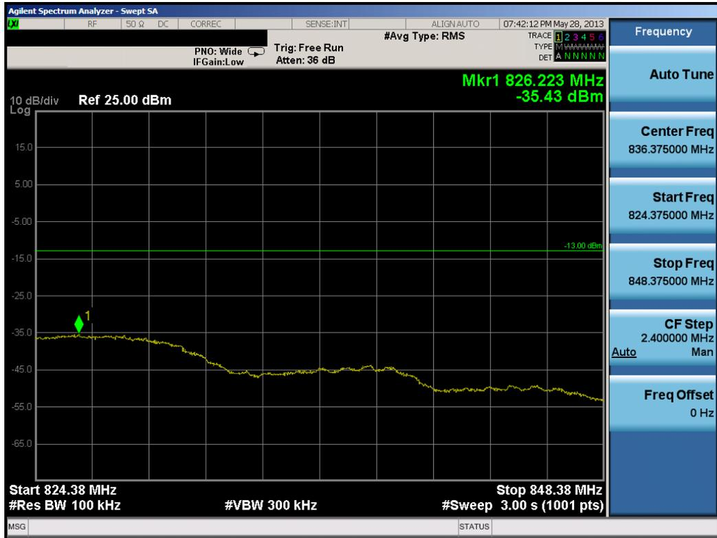
Plot 7-49. Extended Band Edge Plot (10MHz QPSK – RB Size 50)
