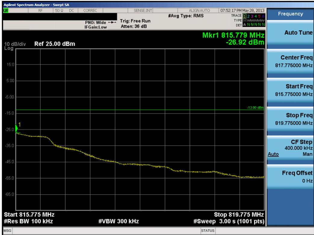
Plot 7-17. Extended Band Edge Plot (1.4MHz QPSK – RB Size 6– Low Channel)
