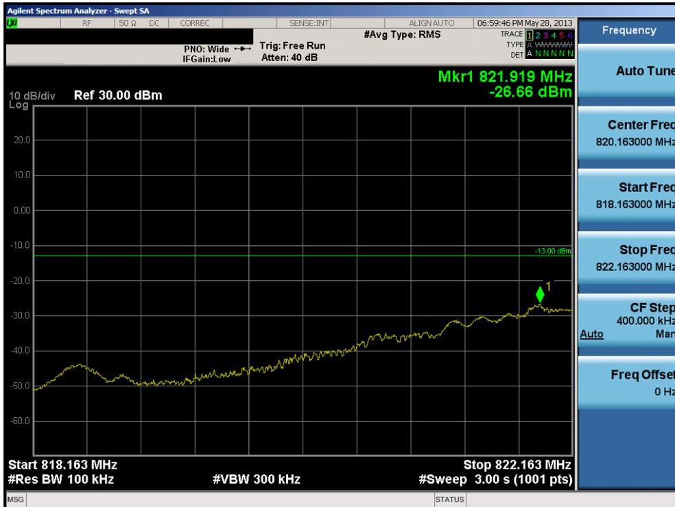
**Plot 7-10. Extended Band Edge Plot – Interior (Ch. 684)**
