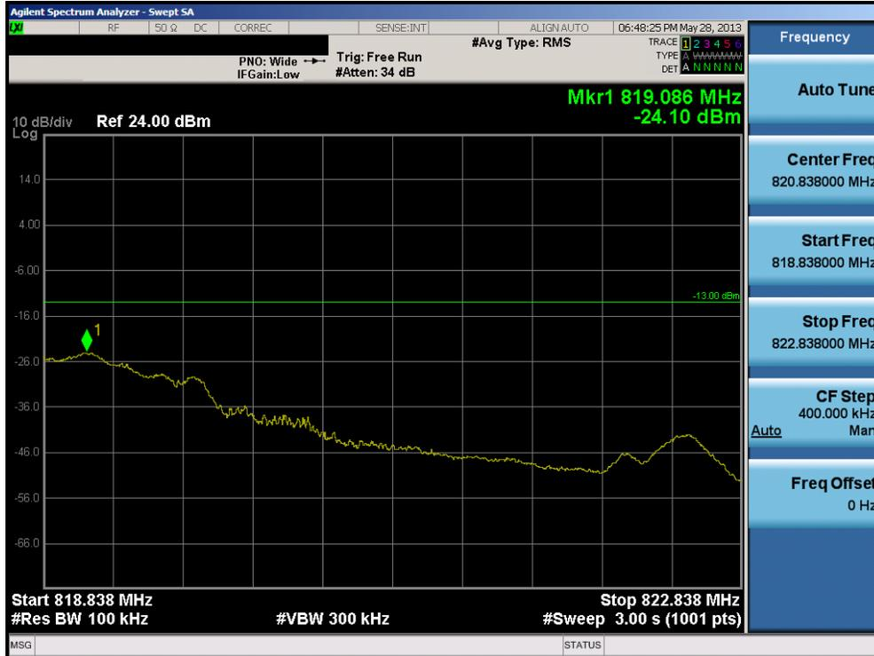
Plot 7-5. Extended Band Edge Plot - Interior (Ch. 476)
