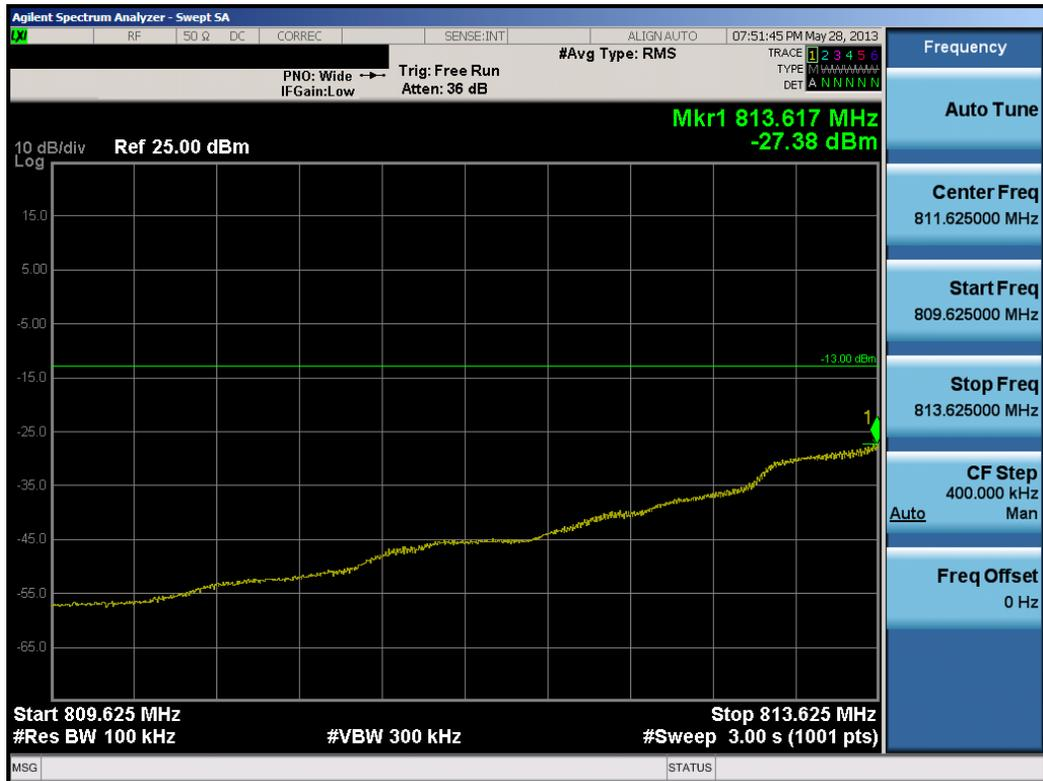
Plot 7-16. Extended Band Edge Plot (1.4MHz QPSK – RB Size 6– Low Channel)
