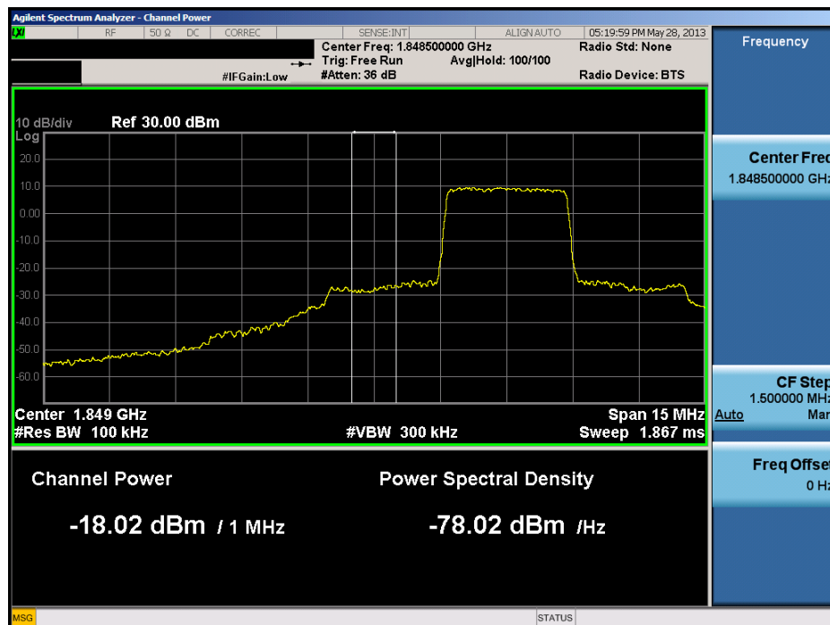
Plot 8-2. Lower Extended Band Edge Plot (3.0MHz QPSK – RB Size 15)
