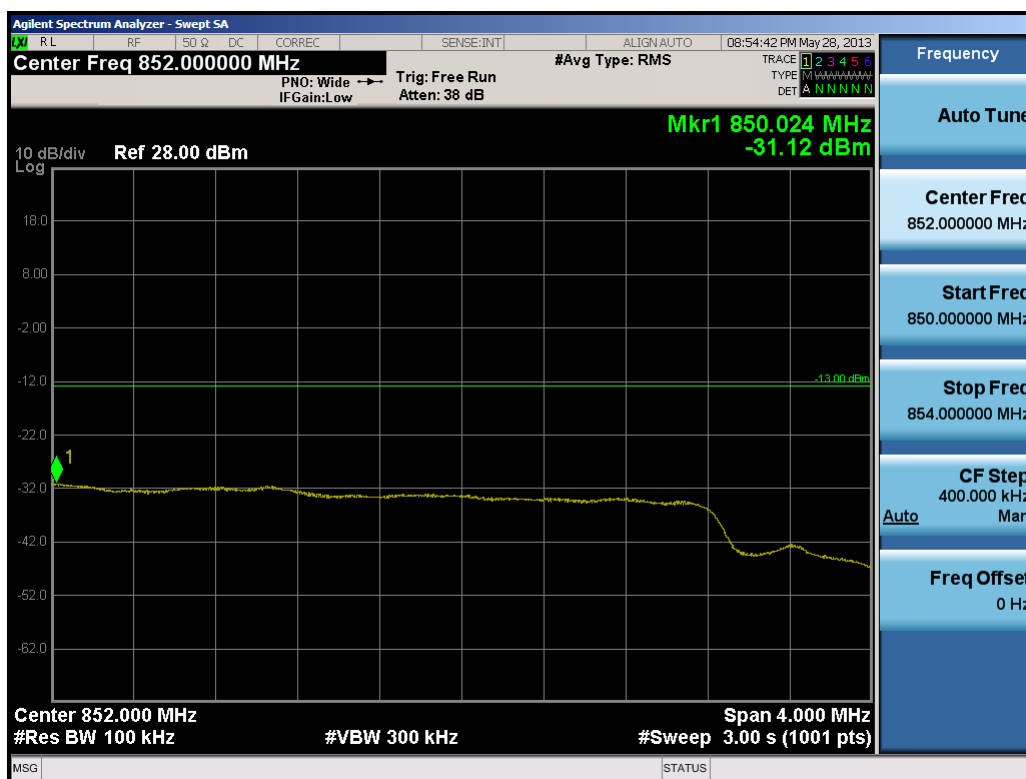
Plot 7-24. Upper Extended Band Edge Plot (5.0MHz QPSK – RB Size 25)
