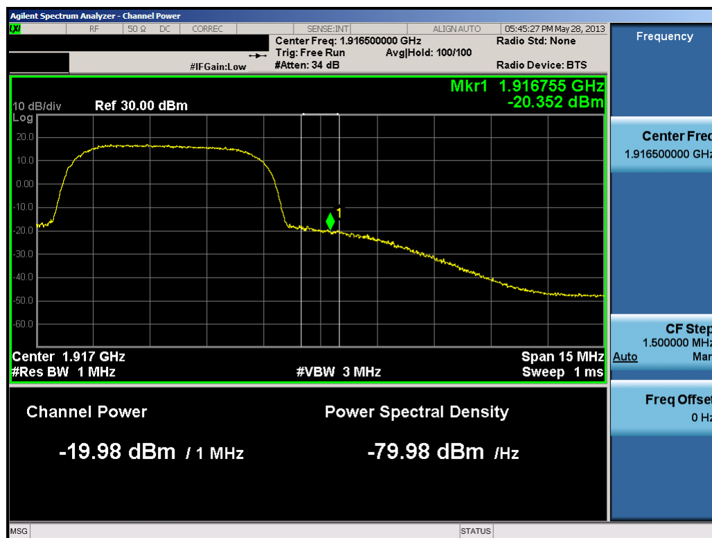
Plot 8-14. Upper Extended Band Edge Plot (5.0MHz QPSK – RB Size 25)
