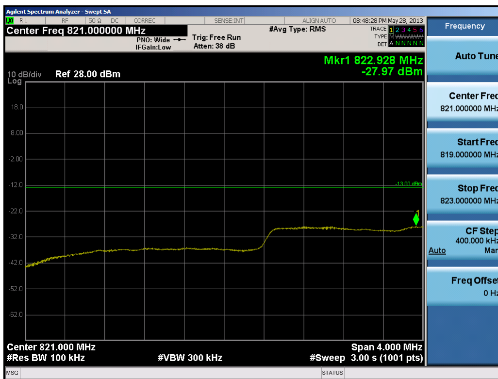
Plot 7-8. Lower Extended Band Edge Plot (3.0MHz QPSK - RB Size 15)
