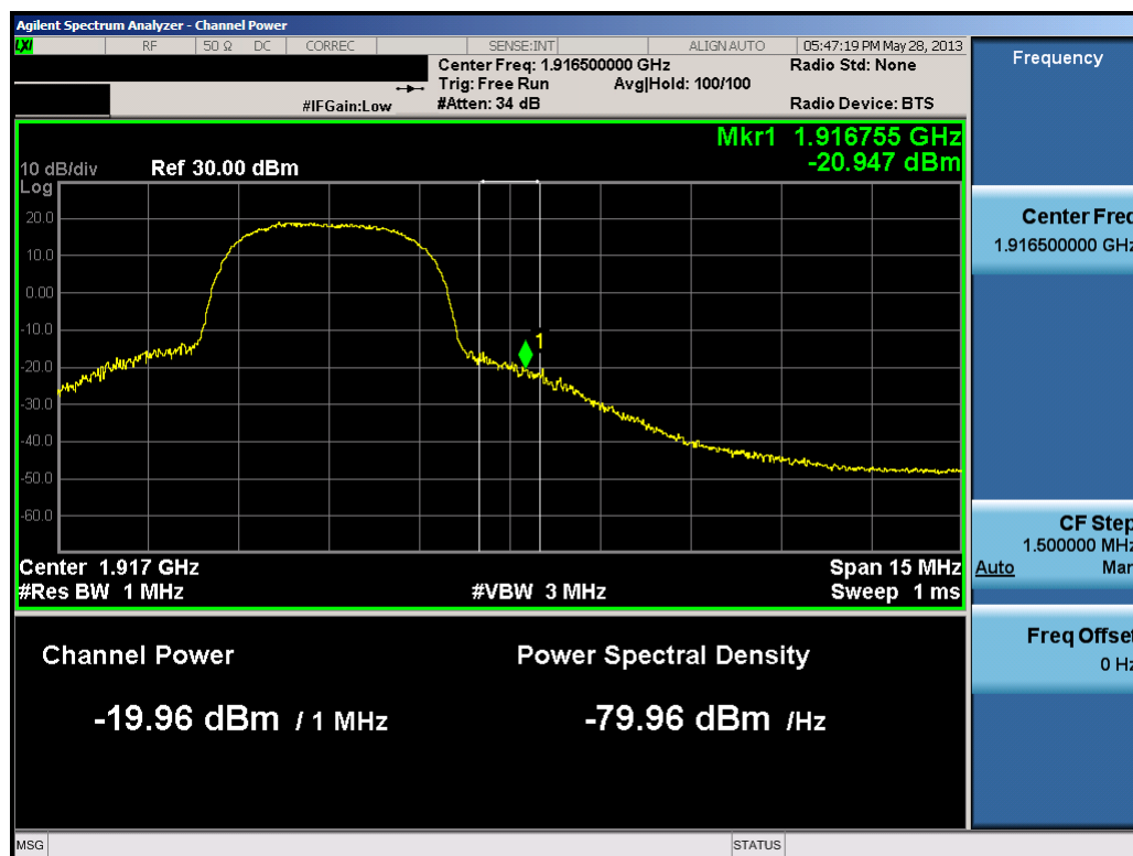
Plot 8-6. Upper Extended Band Edge Plot (3.0MHz QPSK – RB Size 15)
