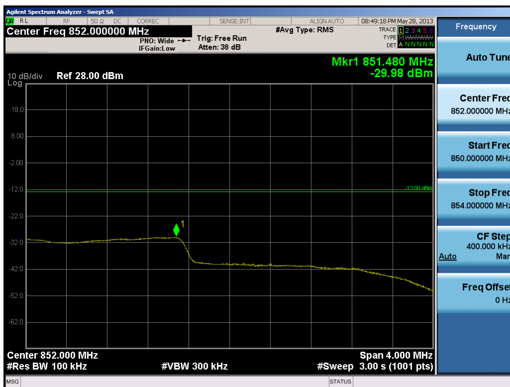
Plot 7-12. Upper Extended Band Edge Plot (3.0MHz QPSK – RB Size 15)
