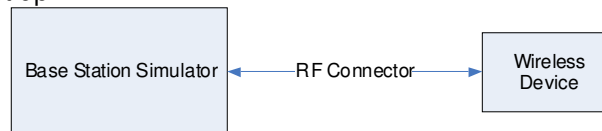
Figure 9-1 Power Measurement Setup
