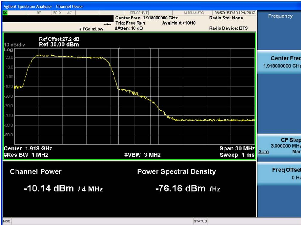
Upper Extended Band Edge Plot (10MHz QPSK - RB Size 25, Offset 12)
