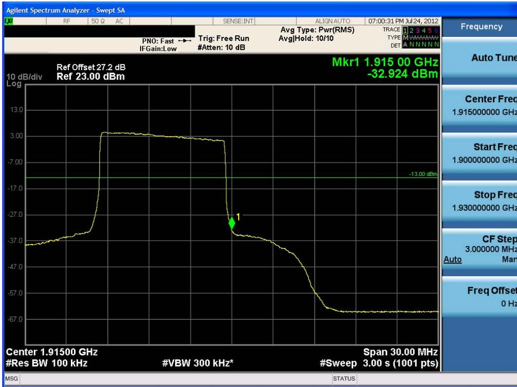
Upper Band Edge Plot (10MHz QPSK - RB Size 25, Offset 12)
