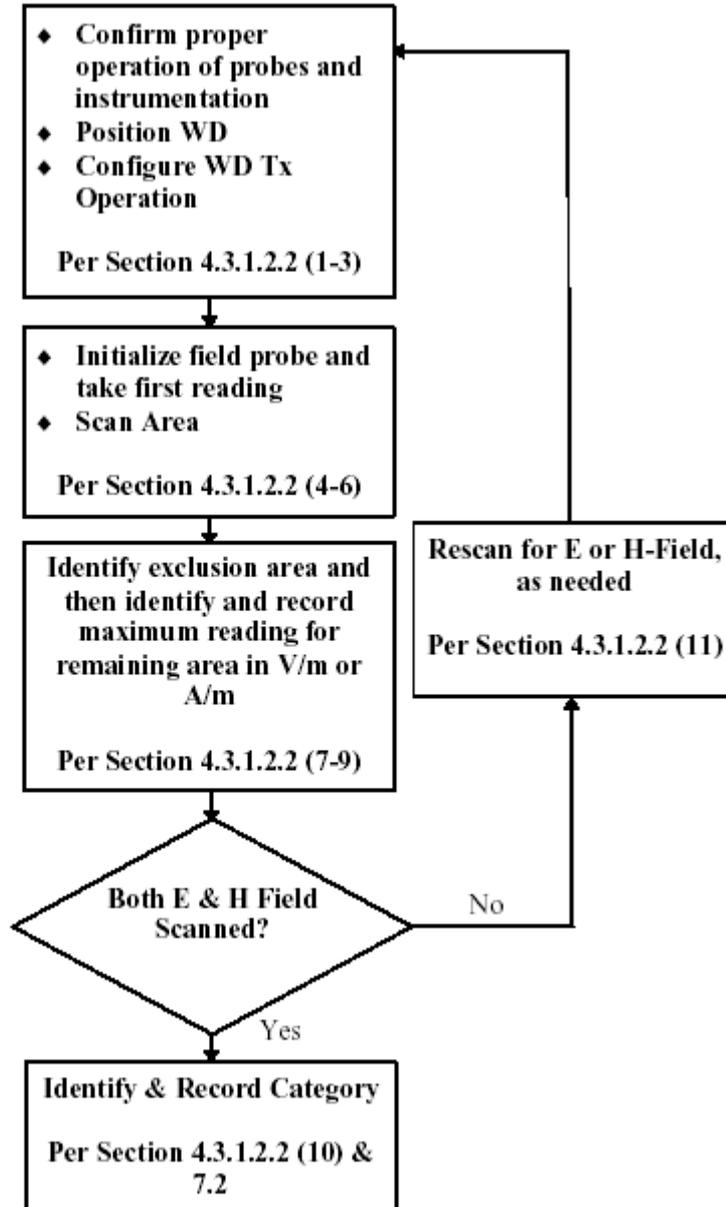
Figure 9. WD near-field emission automated test flowchart
