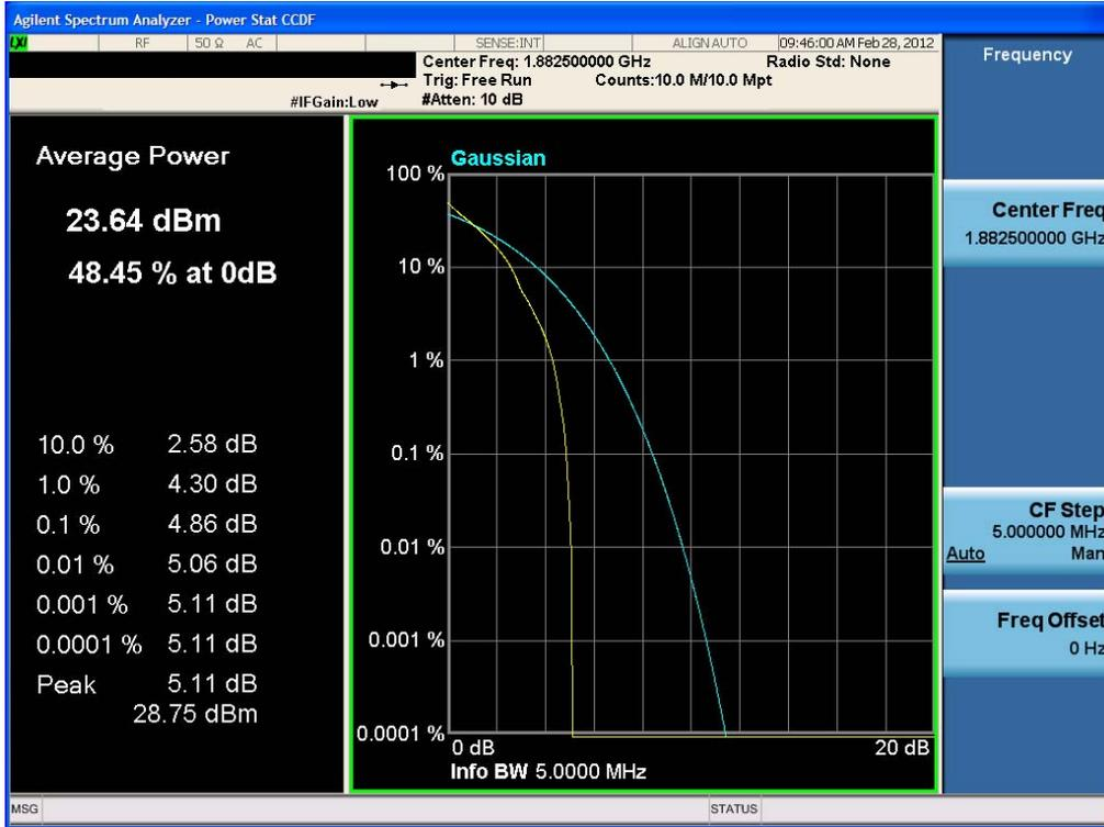
Peak-Average Ratio Plot (5.0 MHz BW, 16-QAM, Band 25: LOW CH)
