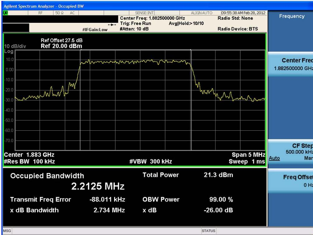
Occupied Bandwidth Plot (5.0 MHz BW, 16-QAM, Band 25: MID CH)
