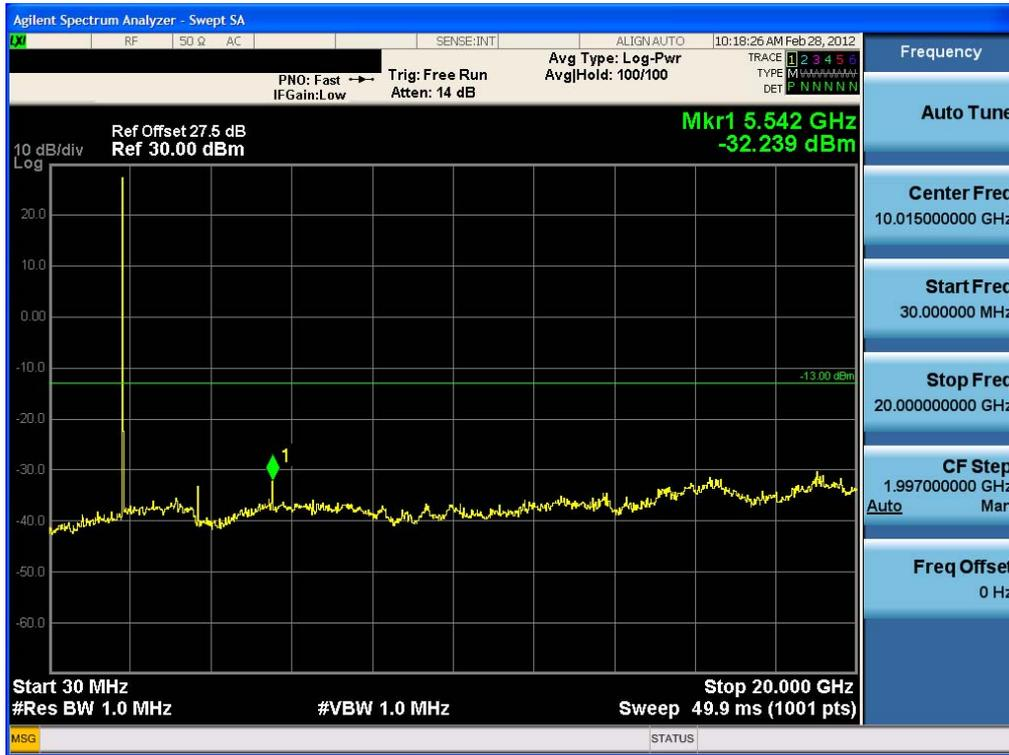
Conducted Spurious Plot (5.0 MHz BW, QPSK, Band 25: LOW CH)
