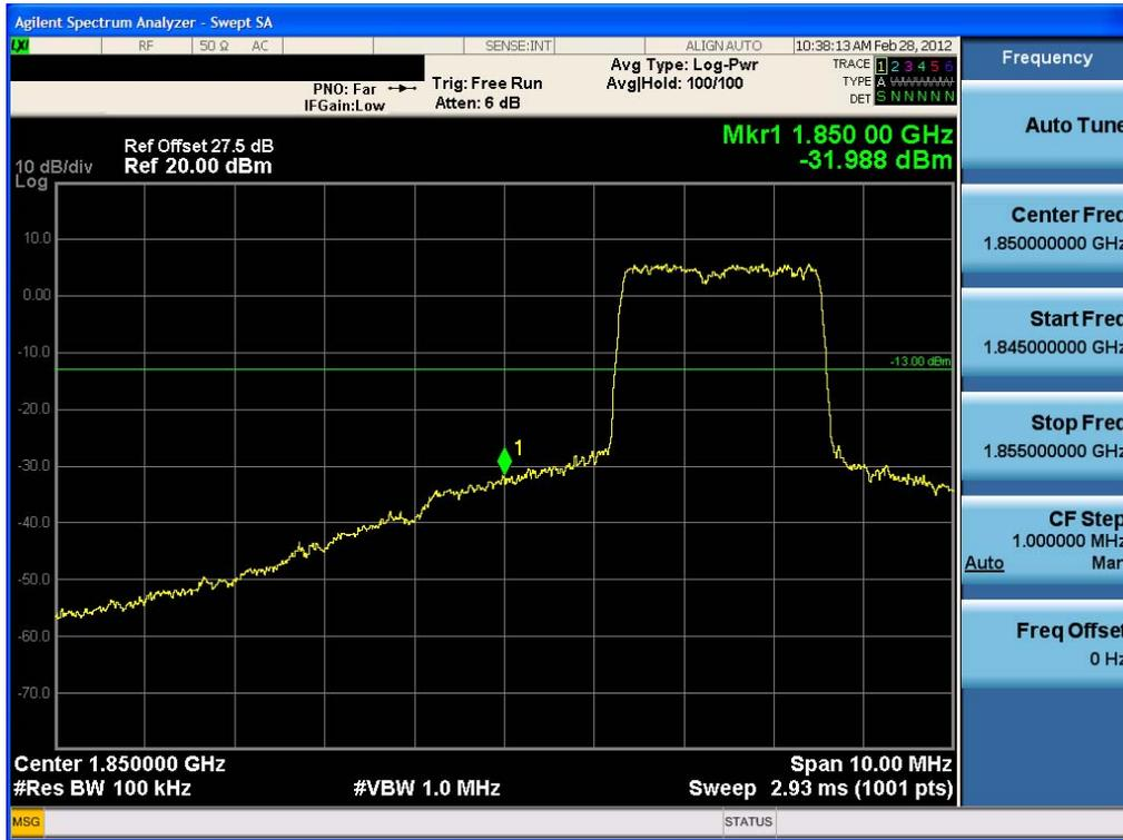
Band Edge Plot (5.0 MHz BW, 16-QAM, Band 25: LOW CH)
