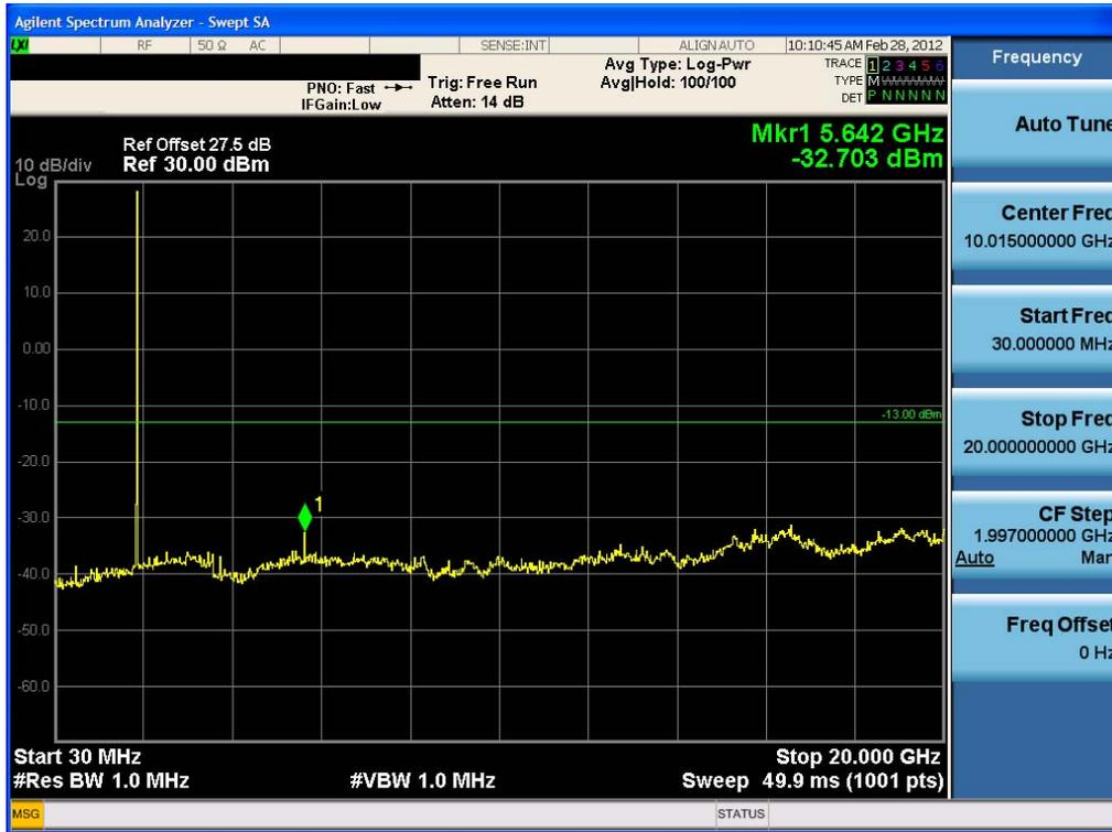
Conducted Spurious Plot (5.0 MHz BW, QPSK, Band 25: MID CH)
