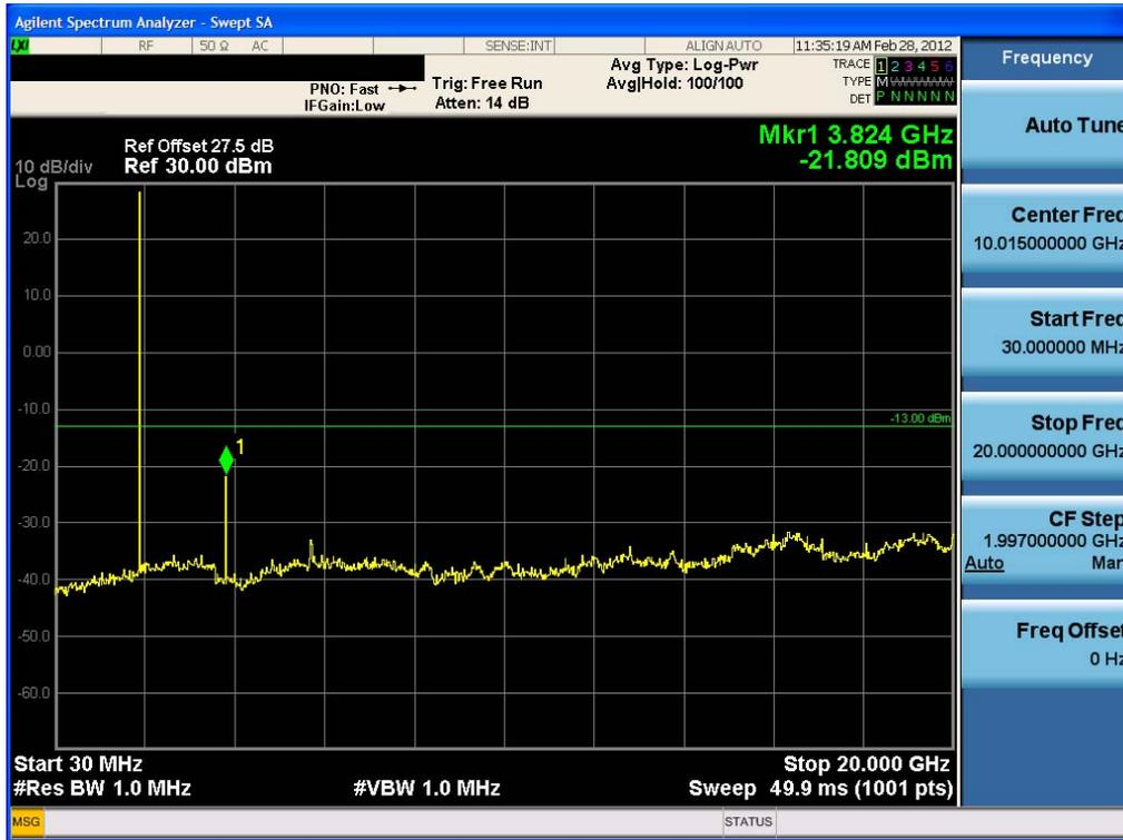
Conducted Spurious Plot (5.0 MHz BW, QPSK, Band 25: HIGH CH)
