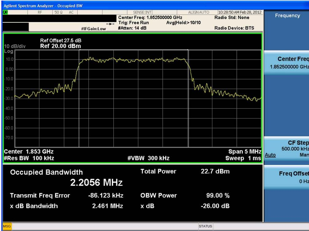
Occupied Bandwidth Plot (5.0 MHz BW, QPSK, Band 25: LOW CH)
