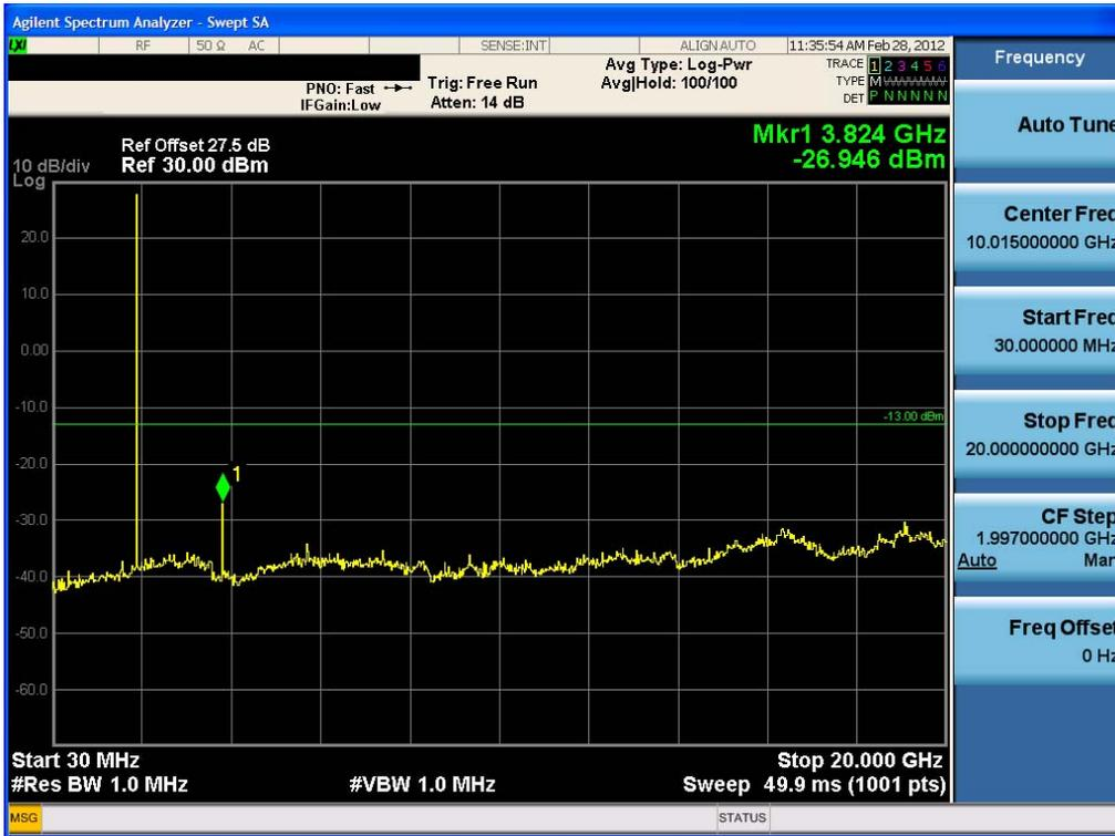
Conducted Spurious Plot (5.0 MHz BW, 16-QAM, Band 25: HIGH CH)
