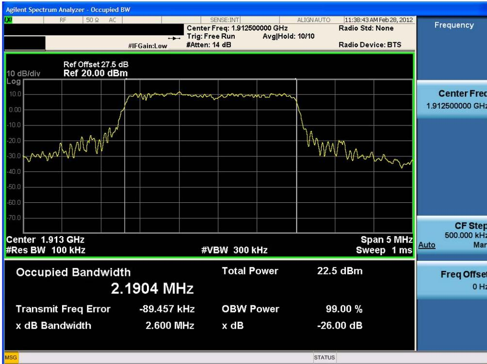
Occupied Bandwidth Plot (5.0 MHz BW, QPSK, Band 25: HIGH CH)
