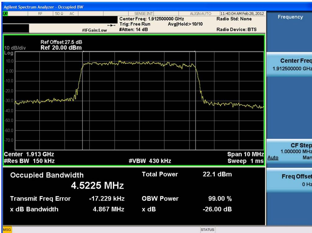
Band Edge Plot (5.0 MHz BW, QPSK, Band 25: LOW CH)
