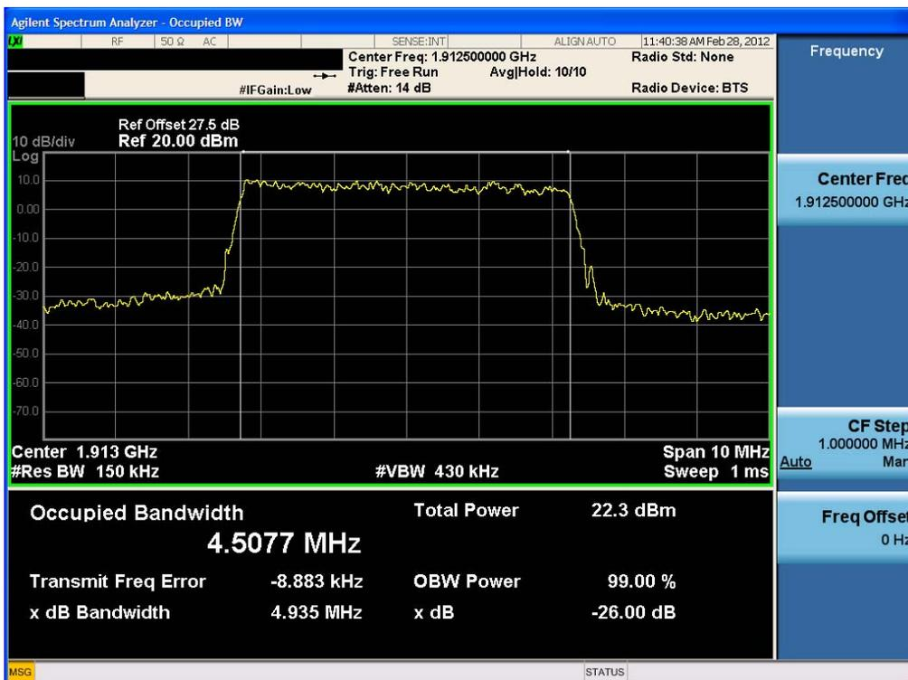
Occupied Bandwidth Plot (5.0 MHz BW, 16-QAM, Band 25: HIGH CH)
