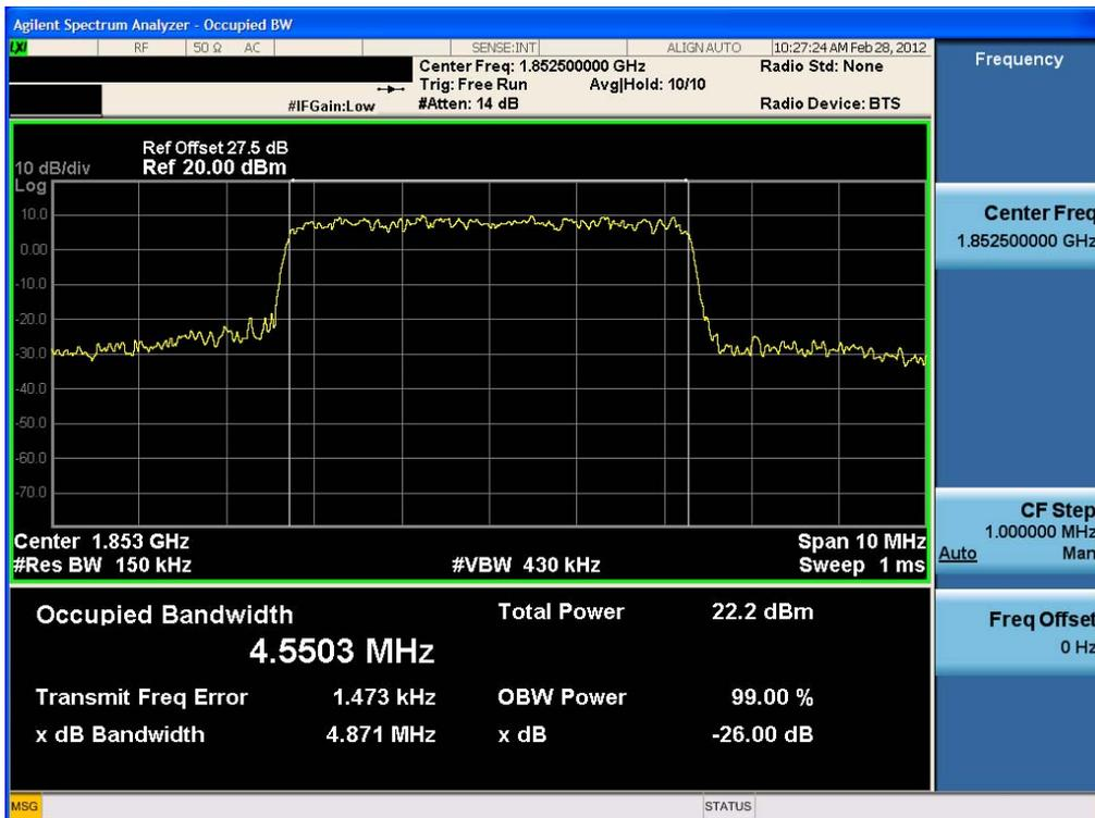
Occupied Bandwidth Plot (5.0 MHz BW, QPSK, Band 25: MID CH)
