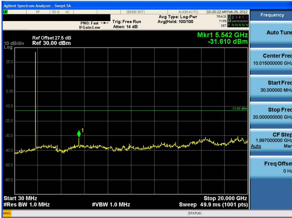
Conducted Spurious Plot (5.0 MHz BW, 16-QAM, Band 25: LOW CH)
