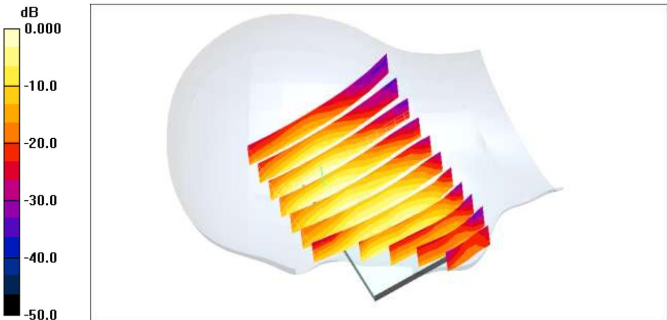
**MultiBand SAR: PCS1900 1xRTT & PCS1900 EVDO & WiFi****DUT: LS840; Type: bar; Serial: #1**
