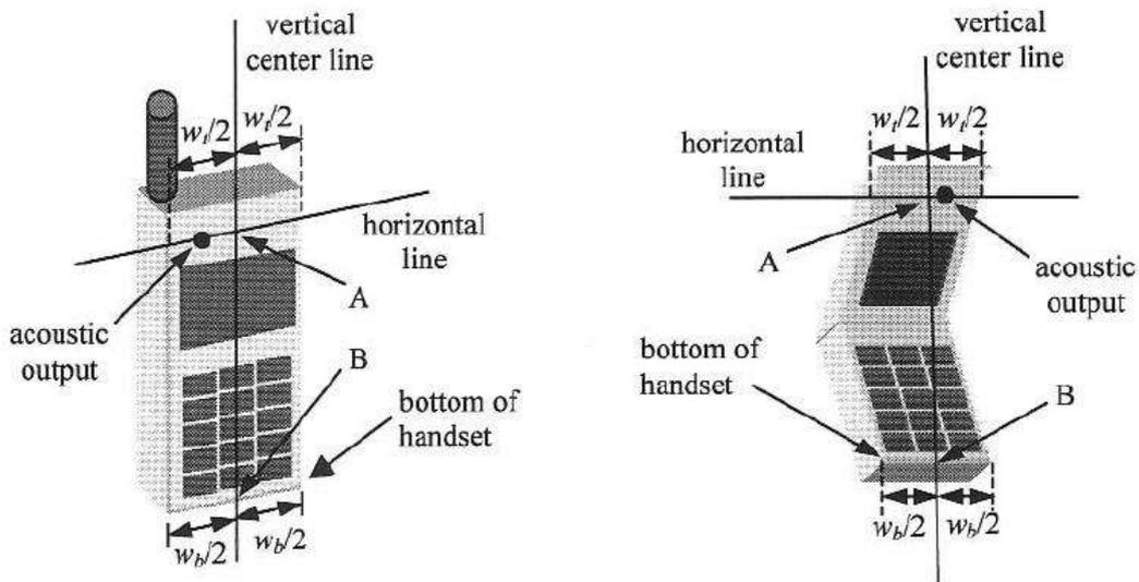
Figure 5.2 Handset vertical and horizontal reference lines
