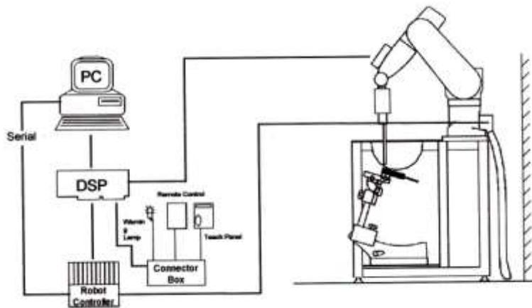
Figure 3.1 HCT SAR Lab. Test Measurement Set-up
