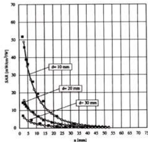
Figure 3.5 E-Field and temperature measurements at 1.8 GHz
