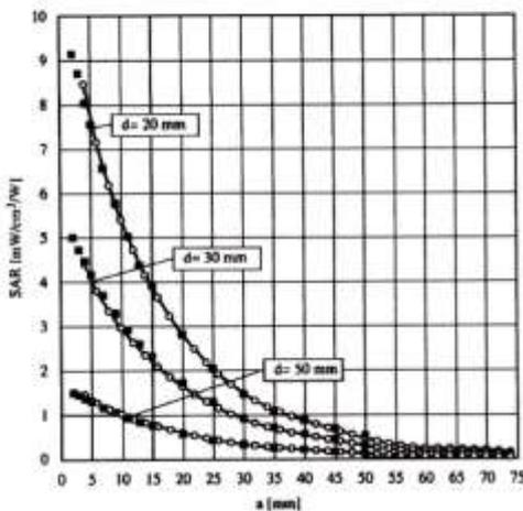
Figure 3.4 E-Field and Temperature measurements at 900 MHz
