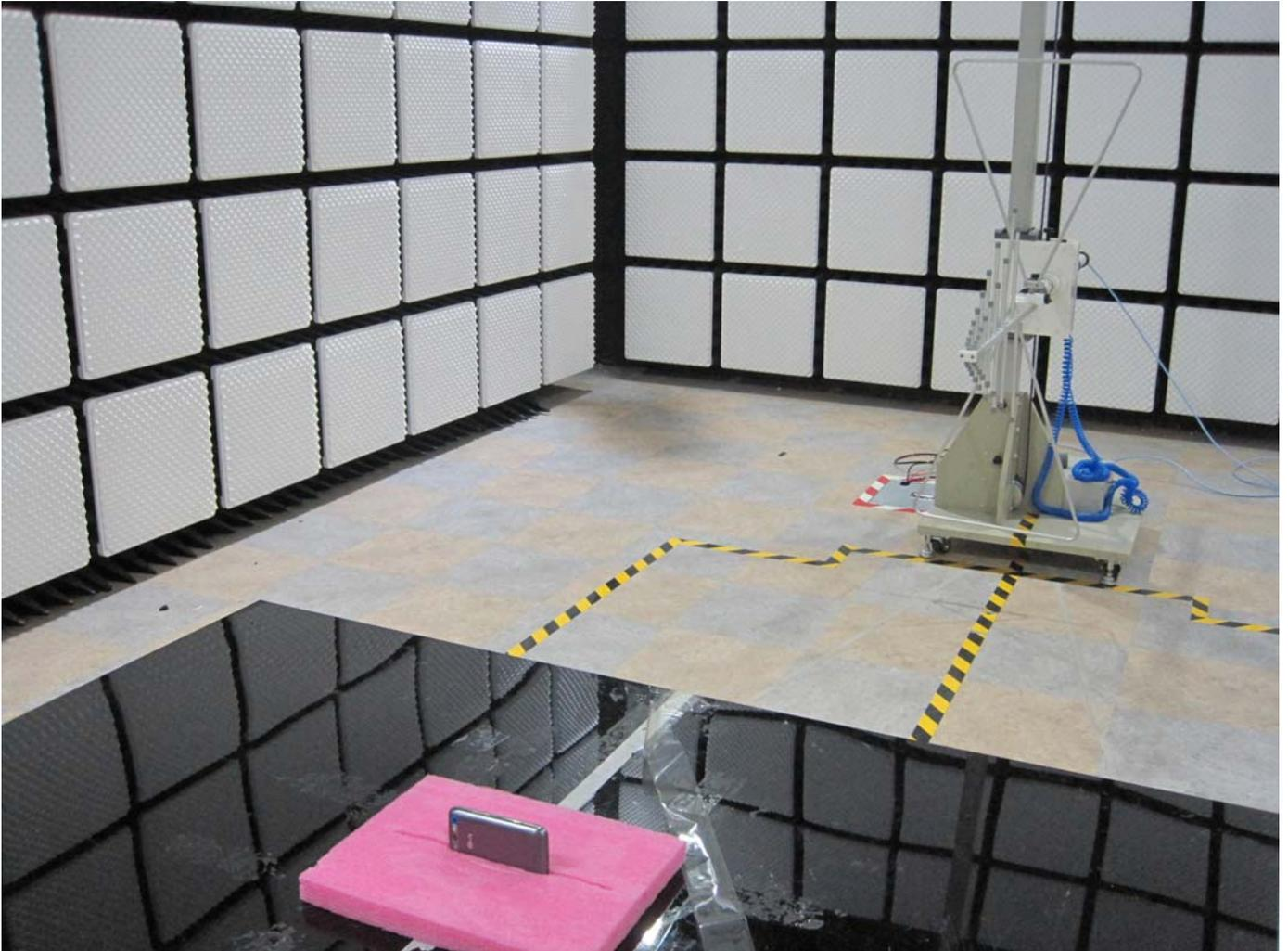
■ BT/WLAN Test Setup Photo
