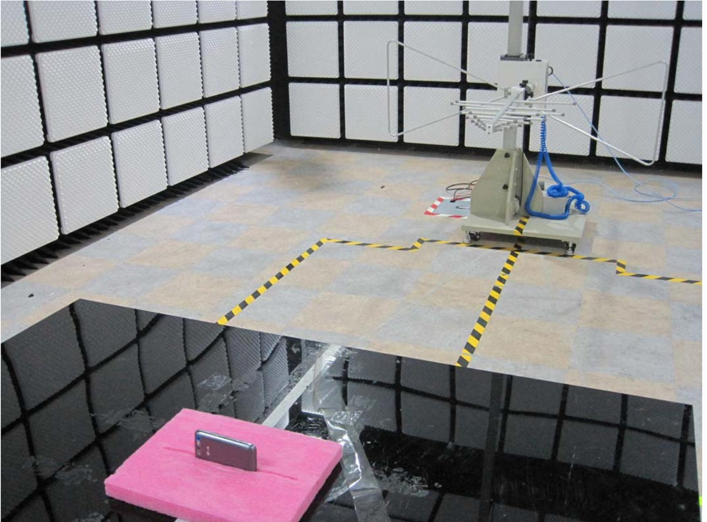
■ BT/WLAN Test Setup Photo
