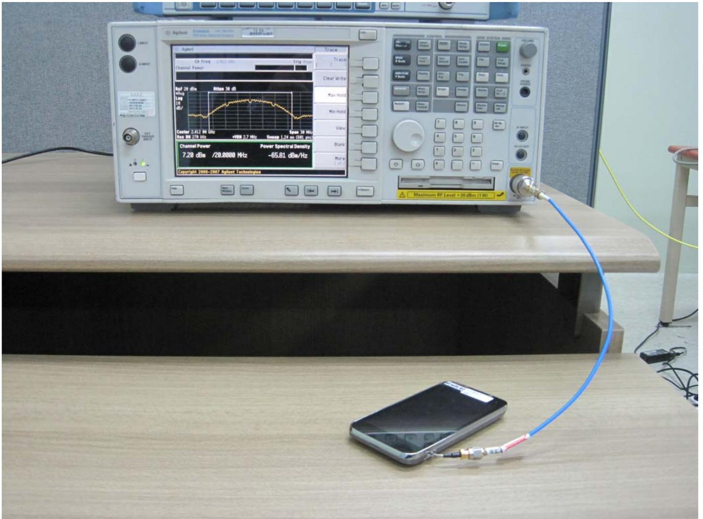
■ Conducted NFC Test Setup Photo
