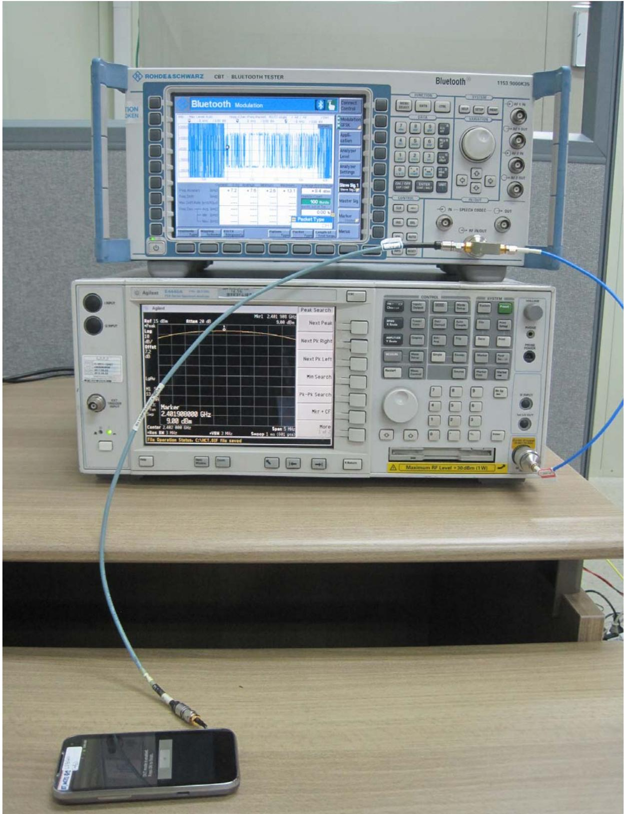
■ Conducted WLAN Test Setup Photo
