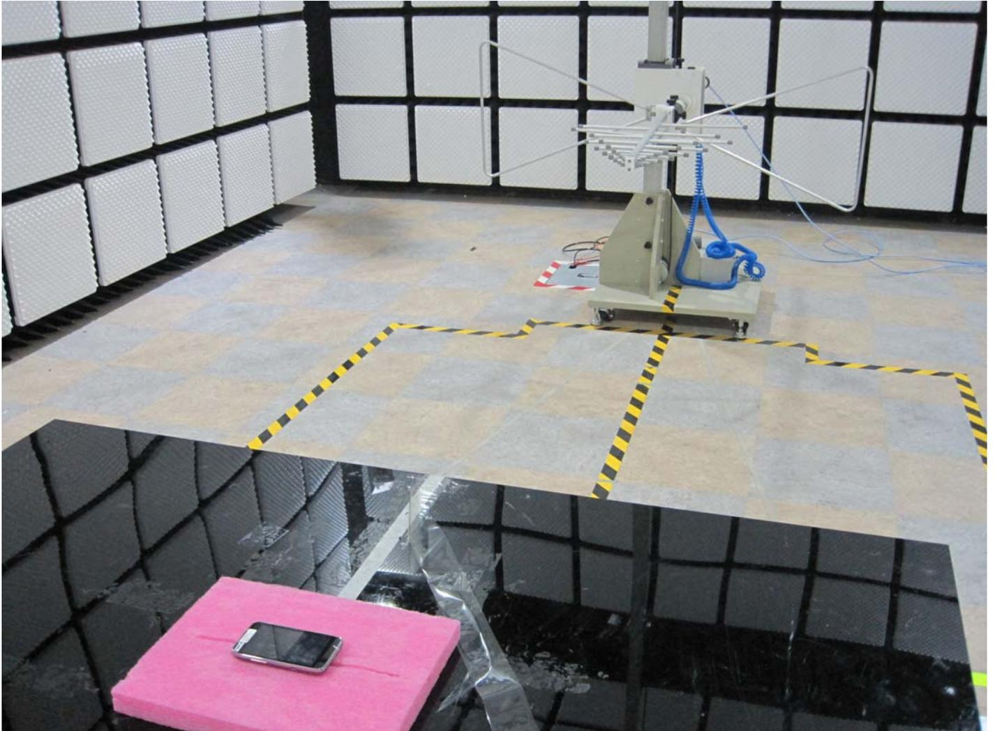
■ BT/WLAN Test Setup Photo
