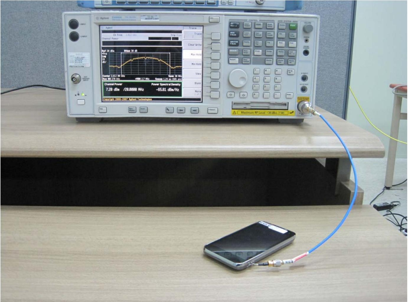
■ Conducted NFC Test Setup Photo
