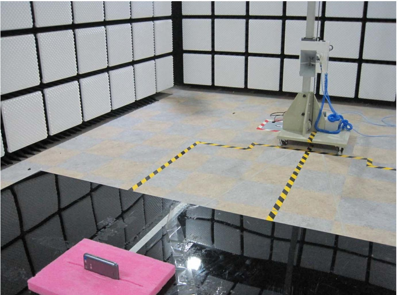
■ BT/WLAN Test Setup Photo
