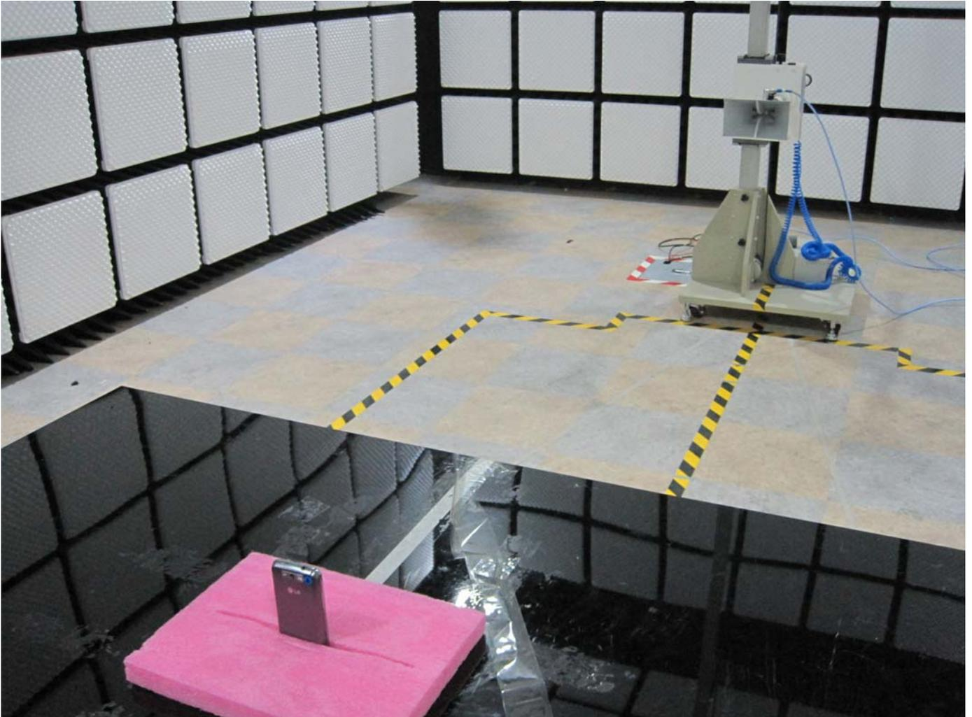
■ BT/WLAN Test Setup Photo
