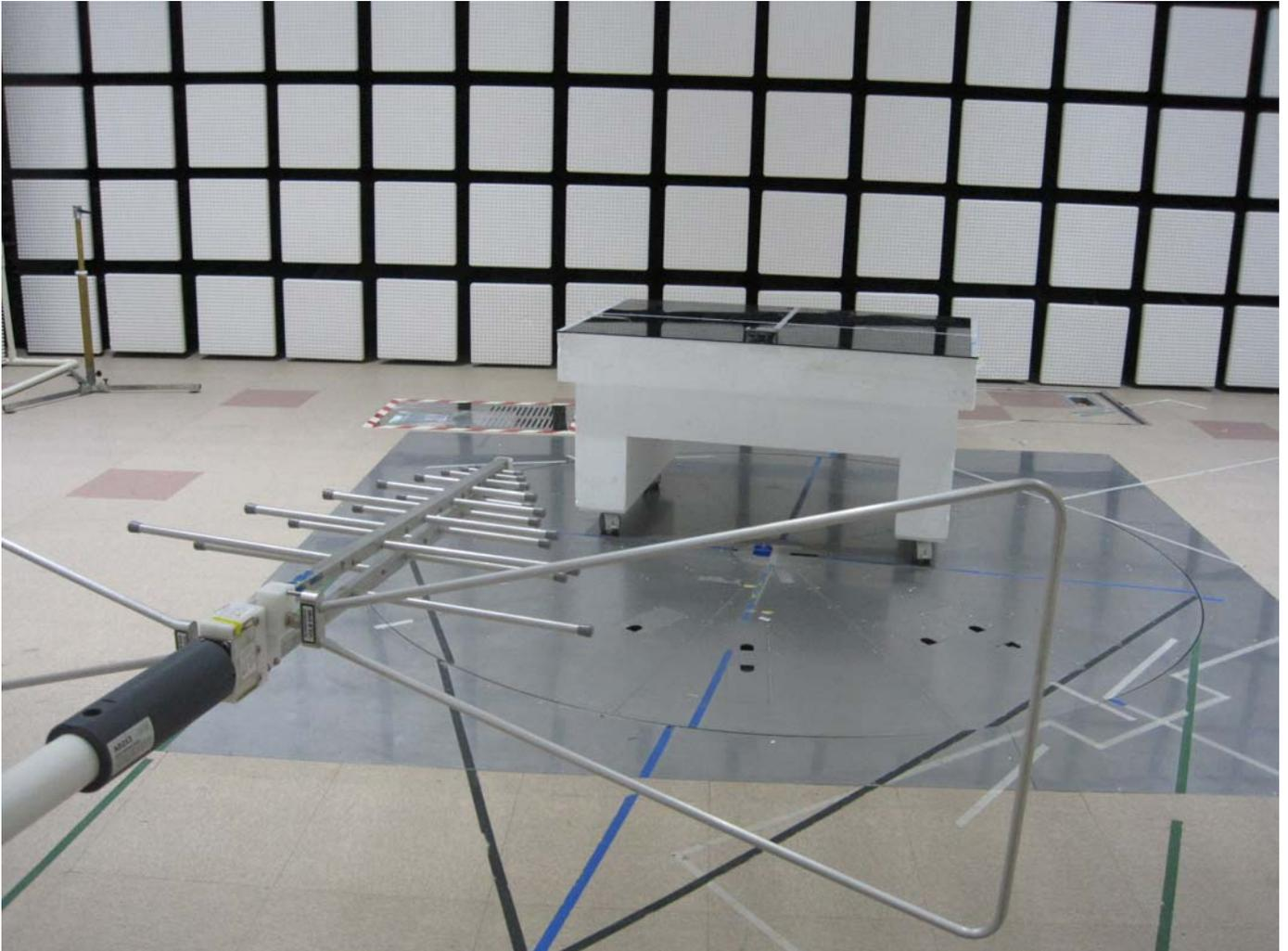
■ BT/WLAN Test Setup Photo
