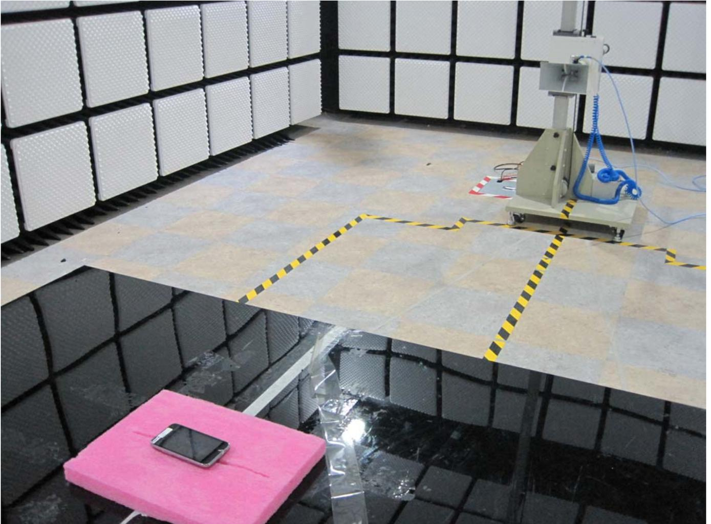
■ BT/WLAN Test Setup Photo
