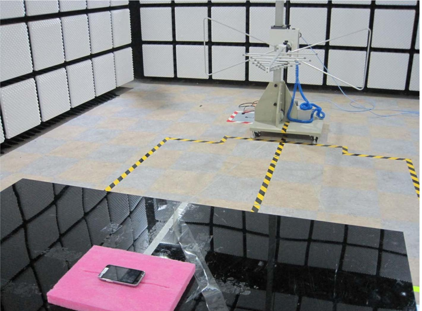
■ BT/WLAN Test Setup Photo
