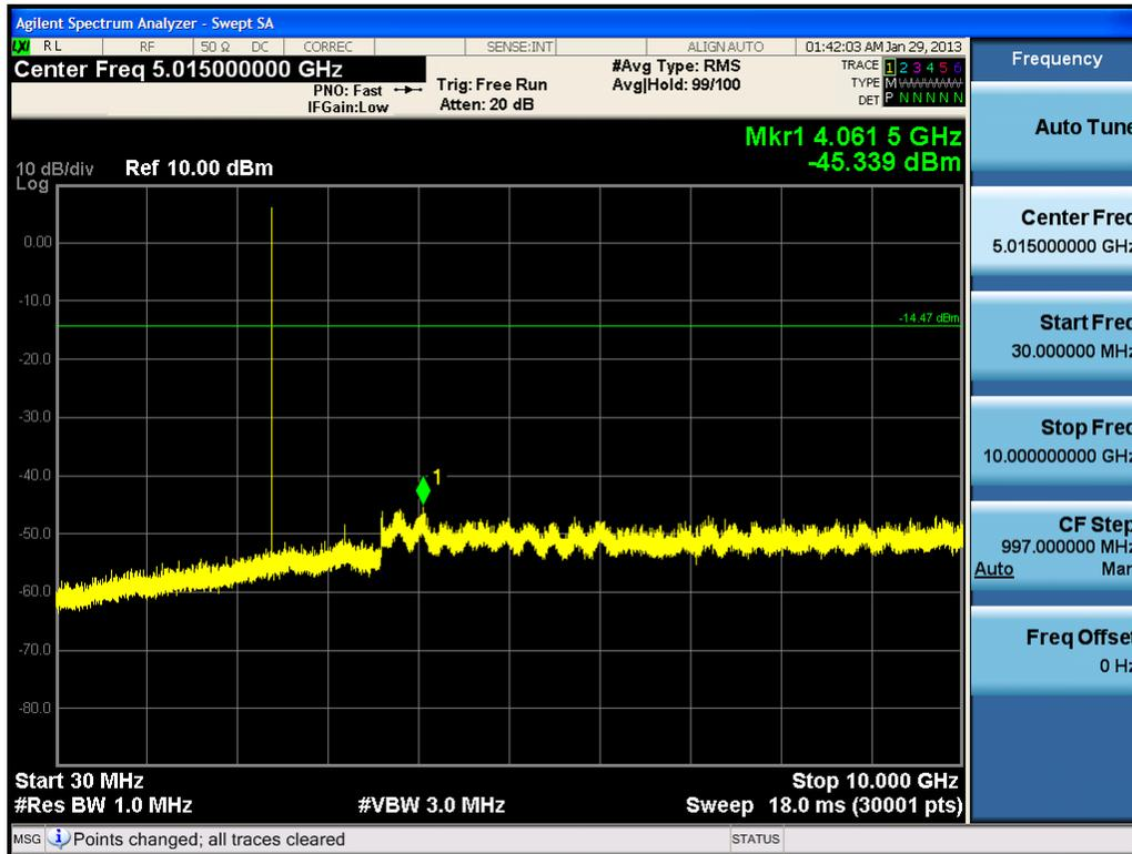
Plot 6-9. Conducted Spurious Plot (Bluetooth (LE) – Ch. 0)
