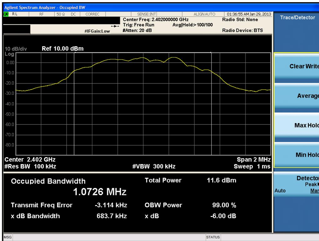
Plot 6-1. 6dB Bandwidth Plot (Bluetooth (LE) – Ch. 0)
