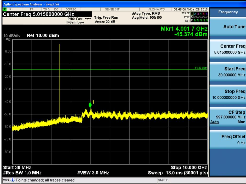
Plot 6-11. Conducted Spurious Plot (Bluetooth (LE) – Ch. 19)
