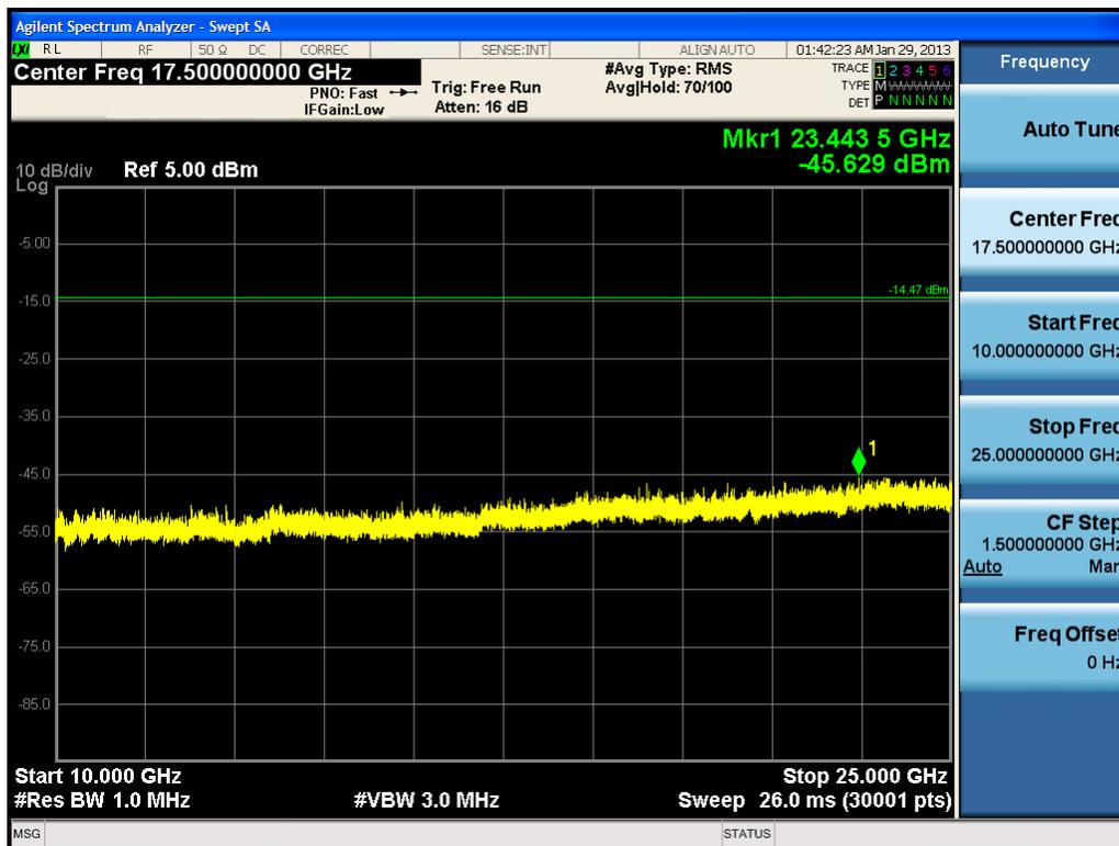
Plot 6-10. Conducted Spurious Plot (Bluetooth (LE) – Ch. 0)
