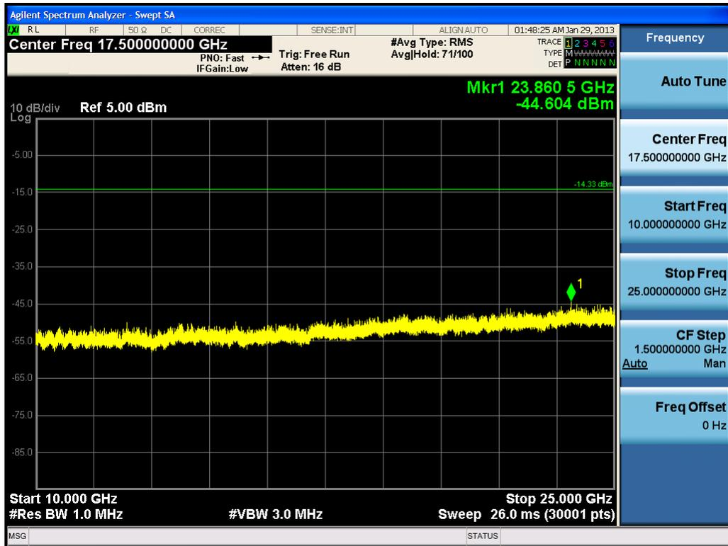
Plot 6-12. Conducted Spurious Plot (Bluetooth (LE) – Ch. 19)
