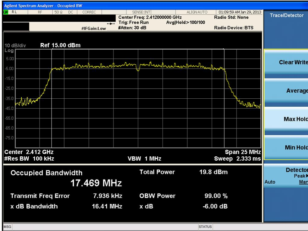
Plot 6-7. 6dB Bandwidth Plot (802.11n (2.4GHz) – Ch. 1)
