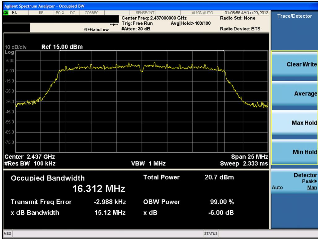
Plot 6-5. 6dB Bandwidth Plot (802.11g – Ch. 6)
