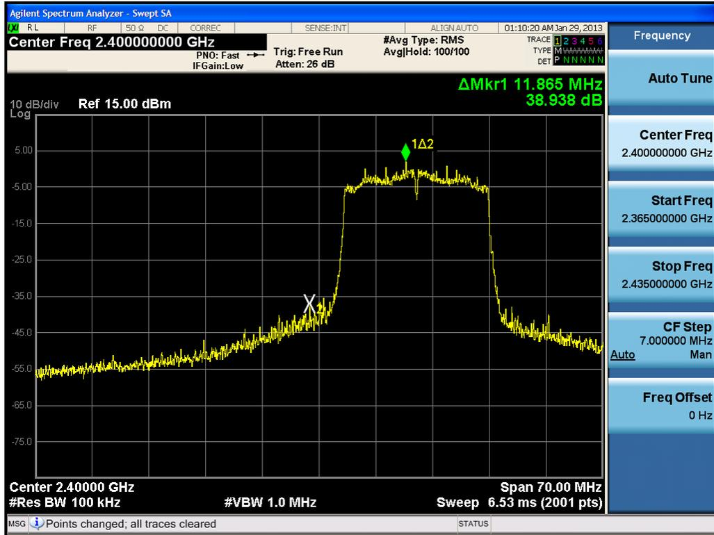
Plot 6-23. Band Edge Plot (802.11n (2.4GHz) – Ch. 1)
