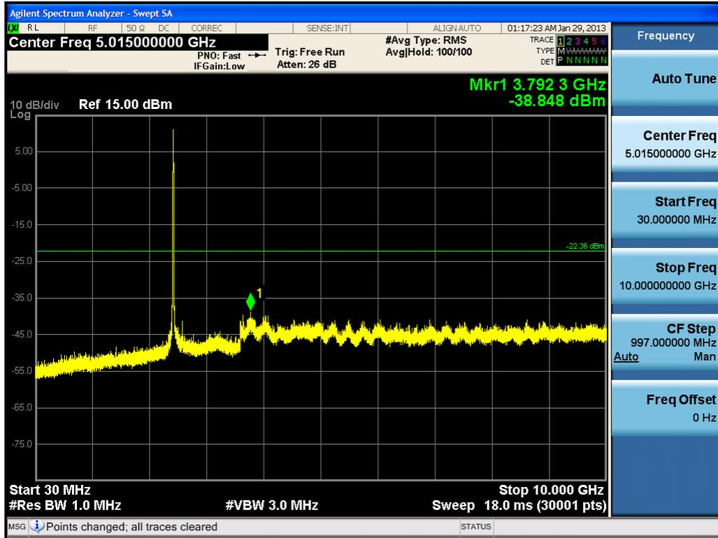
Plot 6-27. Conducted Spurious Plot (802.11b – Ch. 6)
