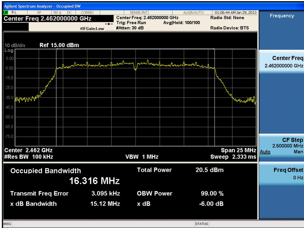
Plot 6-6. 6dB Bandwidth Plot (802.11g – Ch. 11)
