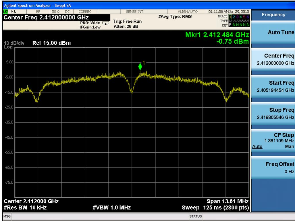
Plot 6-10. Power Spectral Density Plot (802.11b – Ch. 1)
