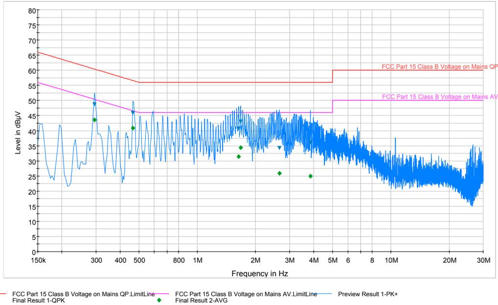
**Plot 6-35. Line Conducted Plot with 802.11b (L1)**
