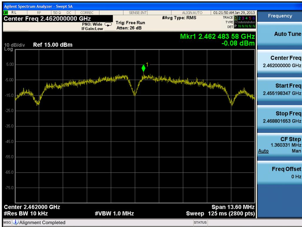
Plot 6-12. Power Spectral Density Plot (802.11b – Ch. 11)
