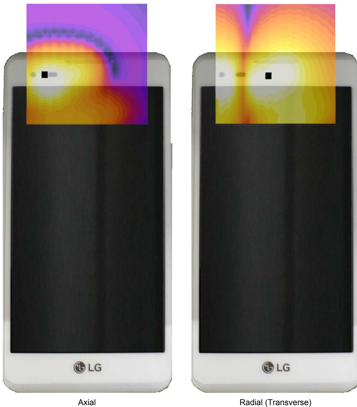
Figure 13-3 T-Coil Scan Overlay Magnetic Field Distributions
