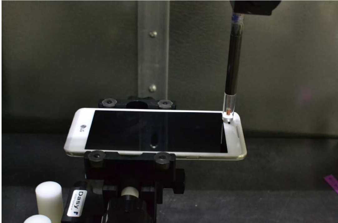
Figure 13-1 Test Setup for Wireless Device
