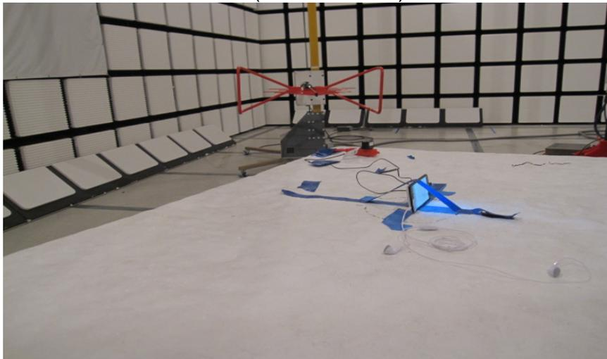
**RADIATED RF MEASUREMENT SETUP (ABOVE 1 GHz)**
