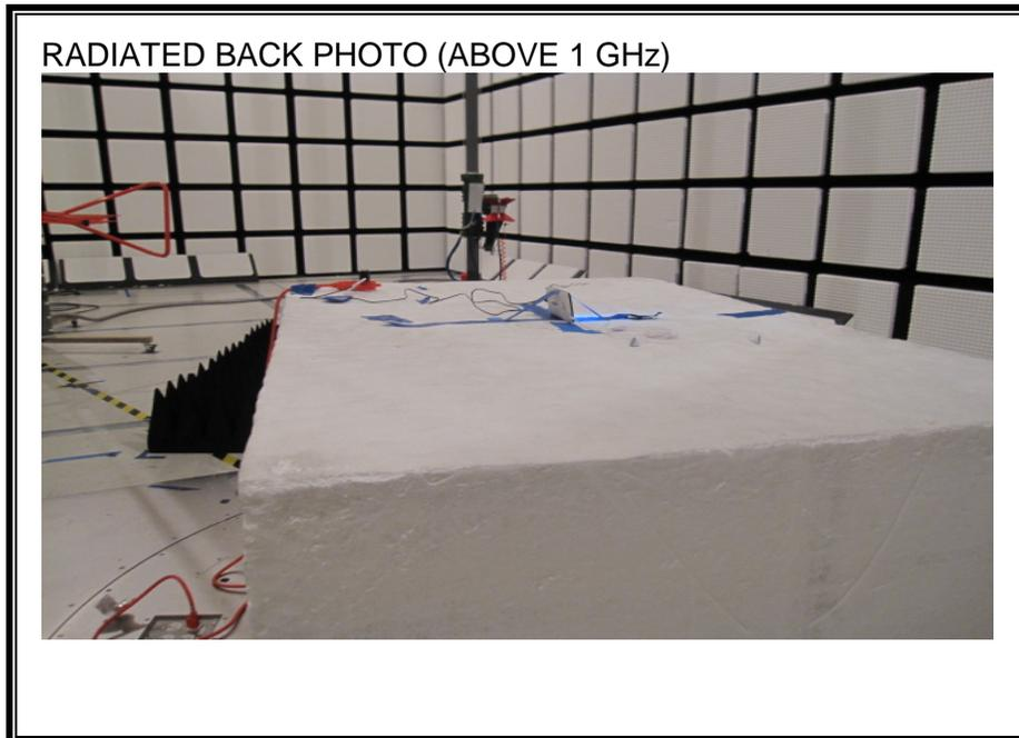
**RADIATED RF MEASUREMENT SETUP FOR PORTABLE CONFIGURATION**
