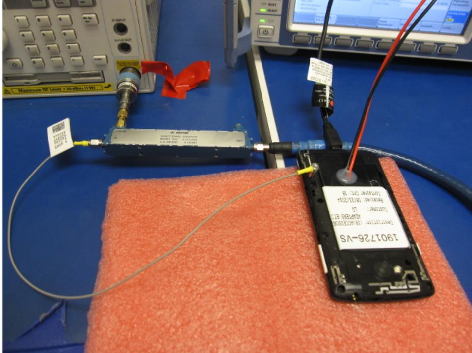
**RADIATED RF MEASUREMENT SETUP FOR PORTABLE CONFIGURATION**
