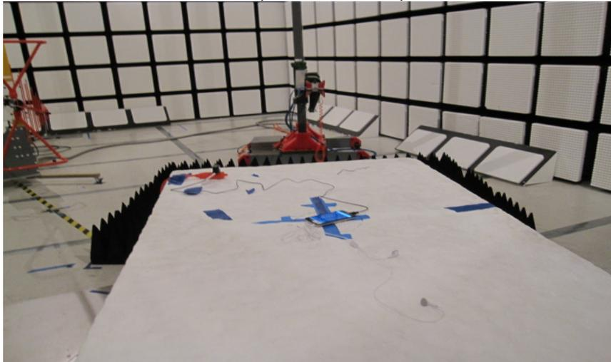
**RADIATED RF MEASUREMENT SETUP FOR PORTABLE CONFIGURATION**
