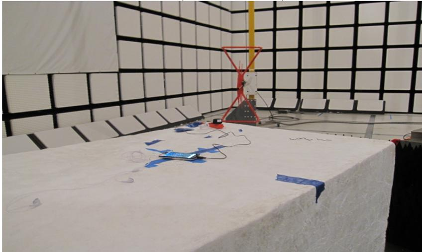
**RADIATED RF MEASUREMENT SETUP (ABOVE 1 GHz)**
