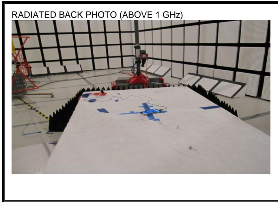
**RADIATED RF MEASUREMENT SETUP FOR PORTABLE CONFIGURATION**
