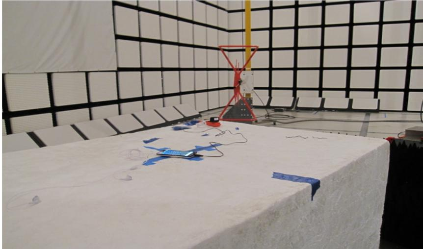
**RADIATED RF MEASUREMENT SETUP (ABOVE 1 GHz)**
