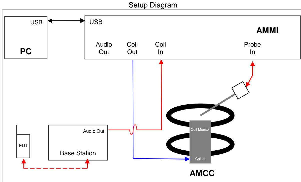
Next step is to measure U, which is the signal from AMMI to the CMU200 during testing. The following setup is used to measure U for narrow band (Voice 1.025 kHz) and broad band (300 Hz – 300 kHz) signals:
