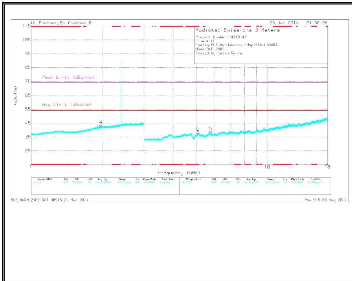
Note: Emission was scanned up to 26GHz; No emissions were detected above the noise floor which was at least 20dB below the specification limit.
