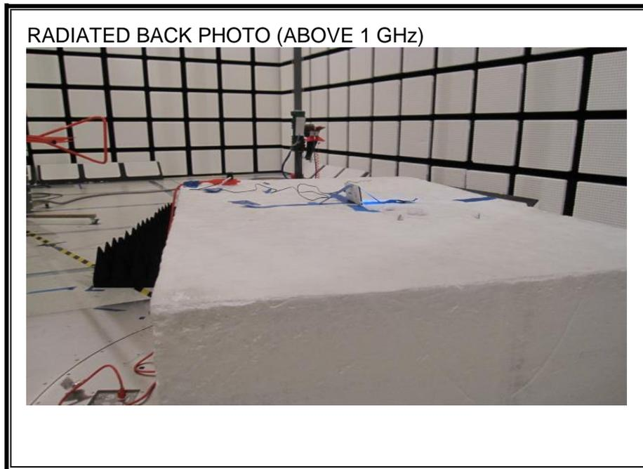
**RADIATED RF MEASUREMENT SETUP FOR PORTABLE CONFIGURATION**
