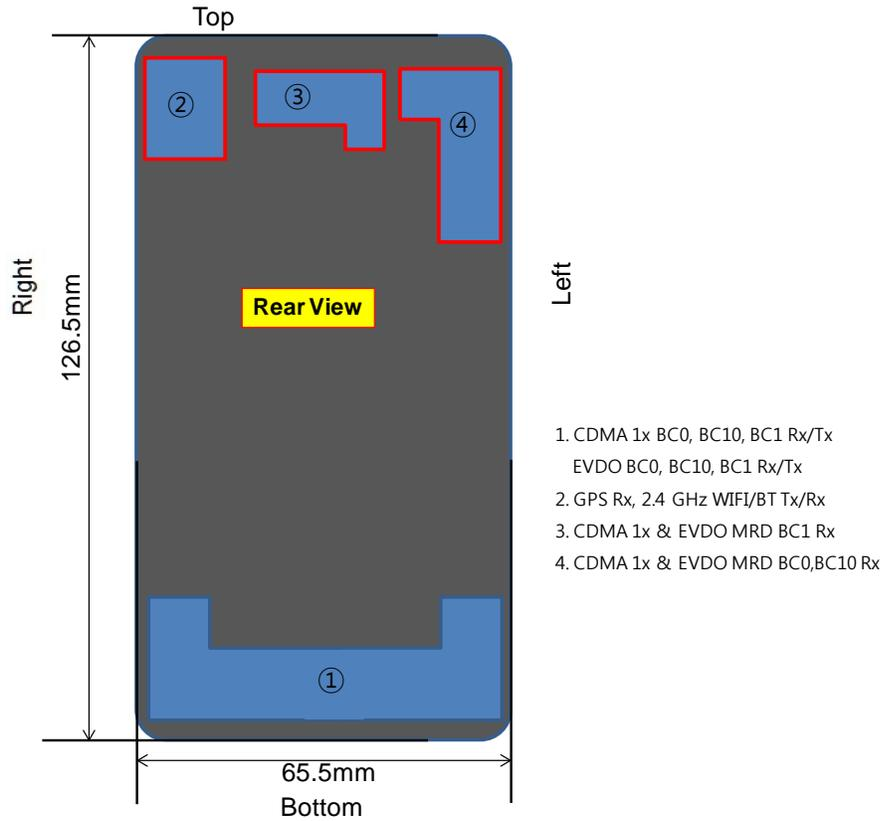
Note: Exact antenna dimensions and separation distances are shown in the Technical Descriptions in the FCC Filing.
