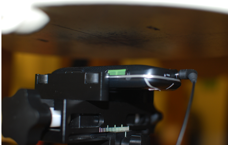
SAR Test Setup Photo 5 – Body-Worn, back side at 2.0 cm
