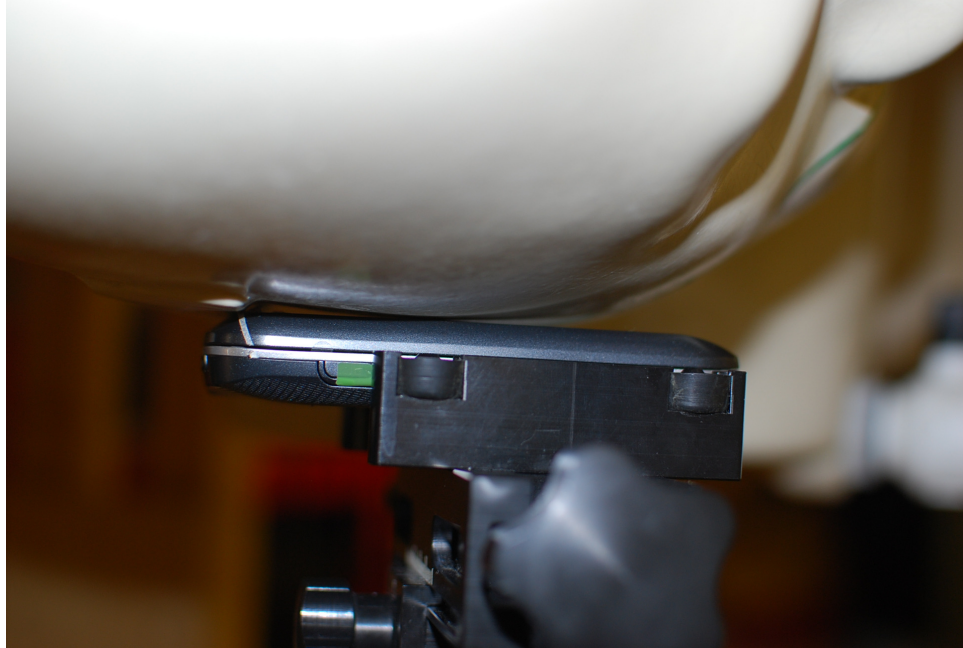
SAR Test Setup Photo 1 – Right Touch
