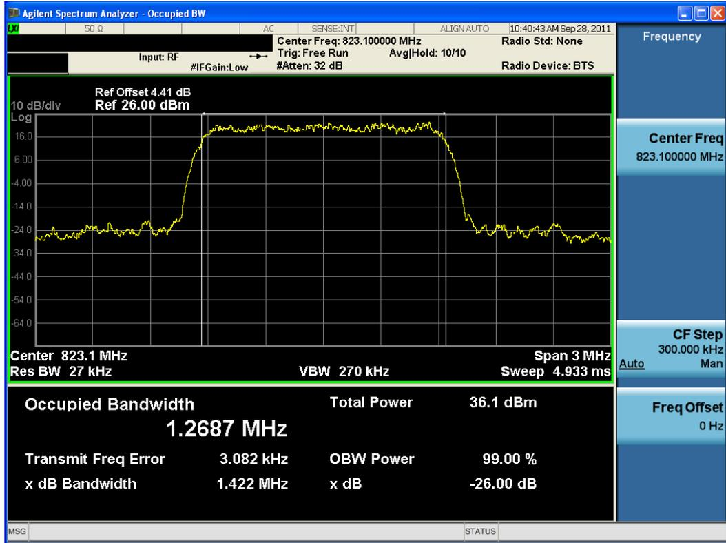
Plot 7-11. Occupied Bandwidth Plot (BC10 CDMA Ch. 684)
