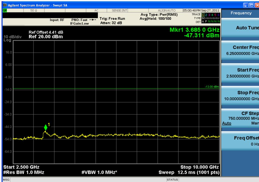
**Plot 7-2. Conducted Spurious Plot (BC10 CDMA Ch. 476)**
