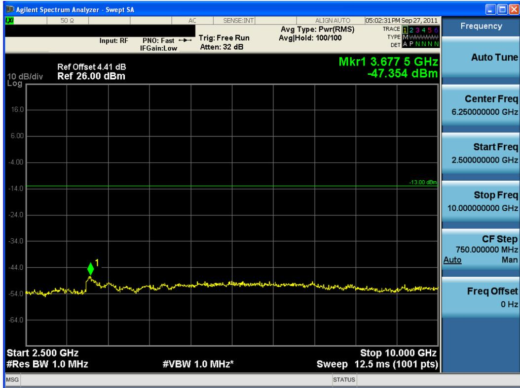
Plot 7-7. Conducted Spurious Plot (BC10 CDMA Ch. 684)
