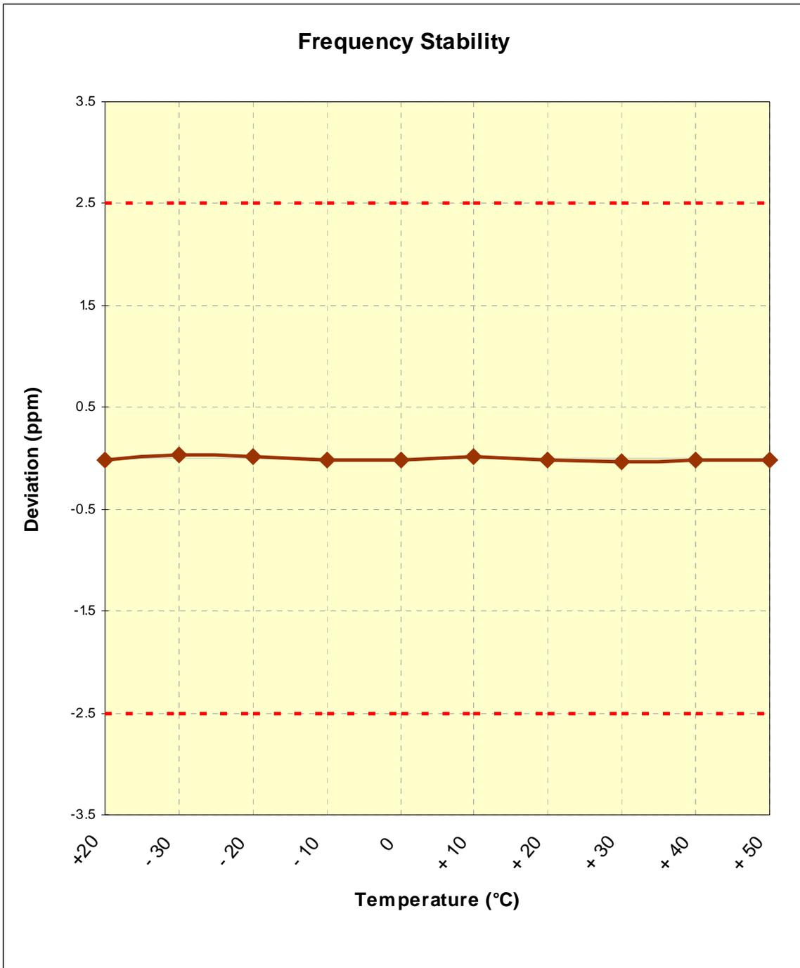
**Figure 6-1. Frequency Stability Graph (Cellular CDMA Mode – Ch. 684)**
