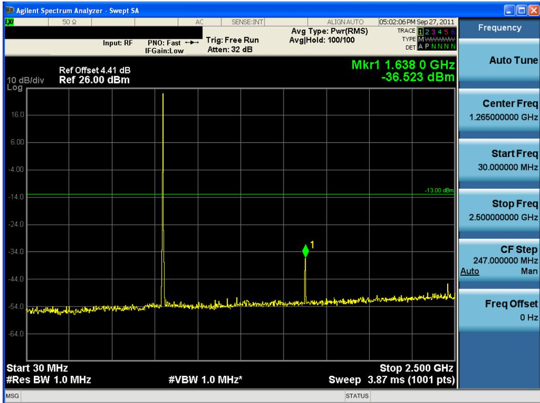
Plot 7-6. Conducted Spurious Plot (BC10 CDMA Ch. 684)
