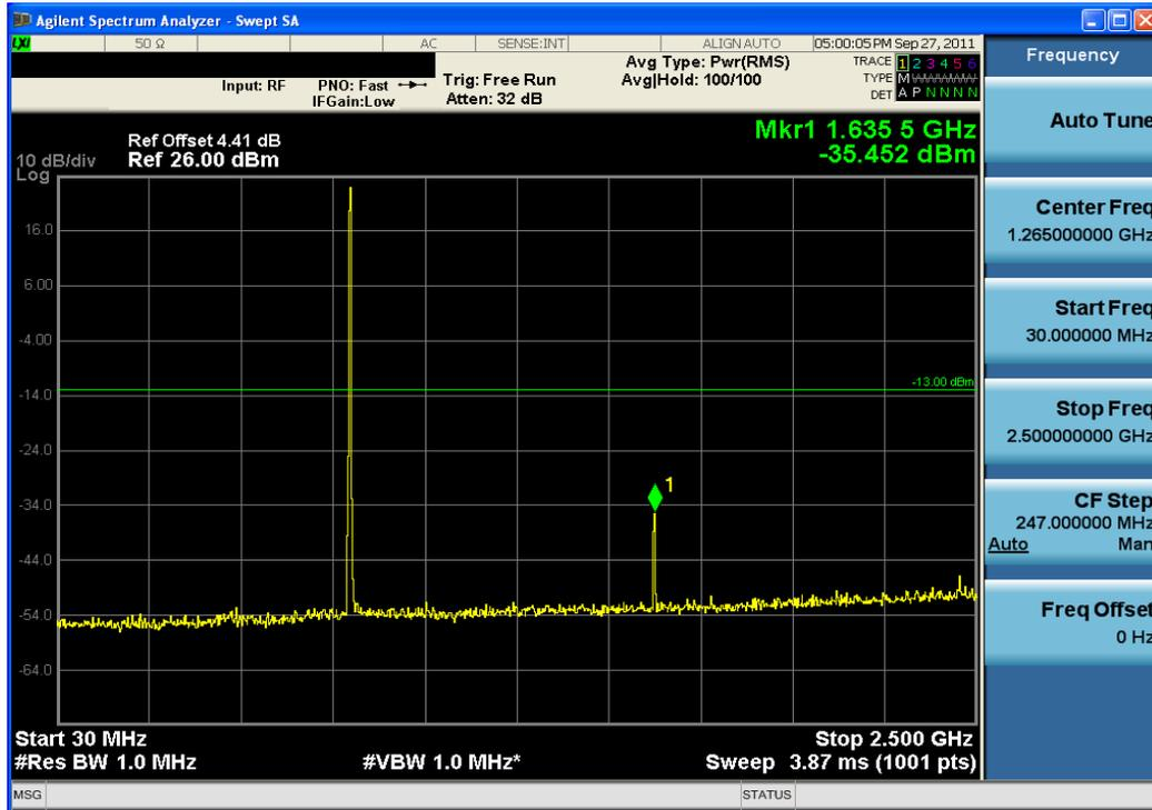
**Plot 7-1. Conducted Spurious Plot (BC10 CDMA Ch. 476)**
