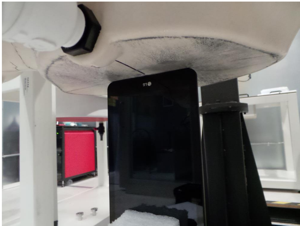
SAR Test Setup Photo 12 – Bottom Edge at 0 mm
