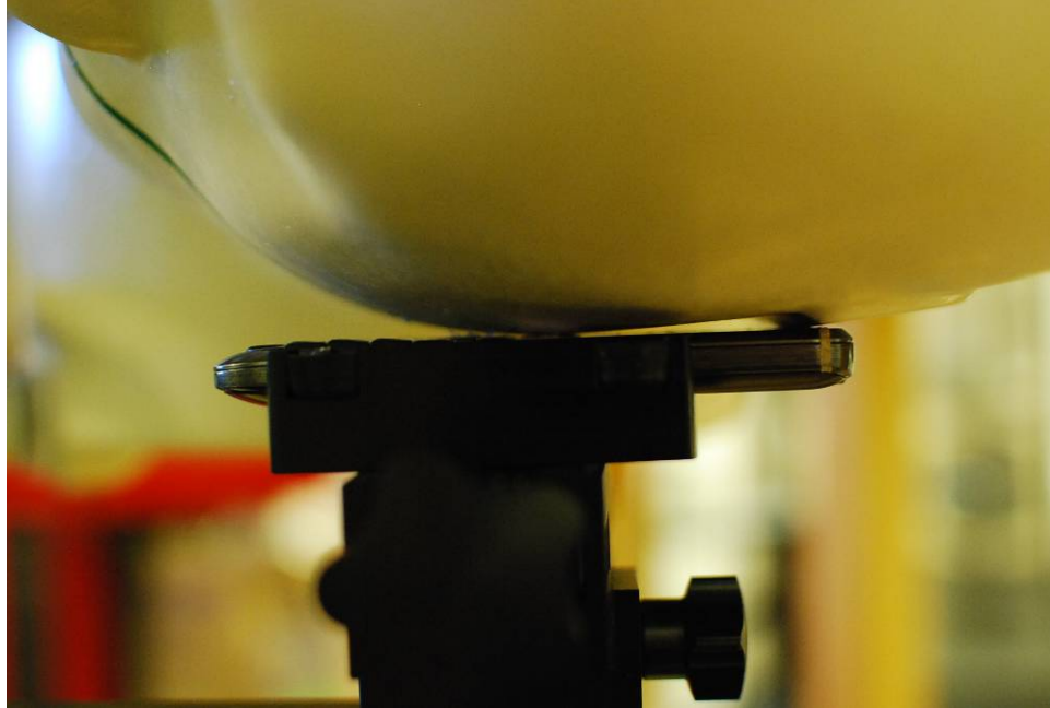
SAR Test Setup Photo 3 – Left Touch
