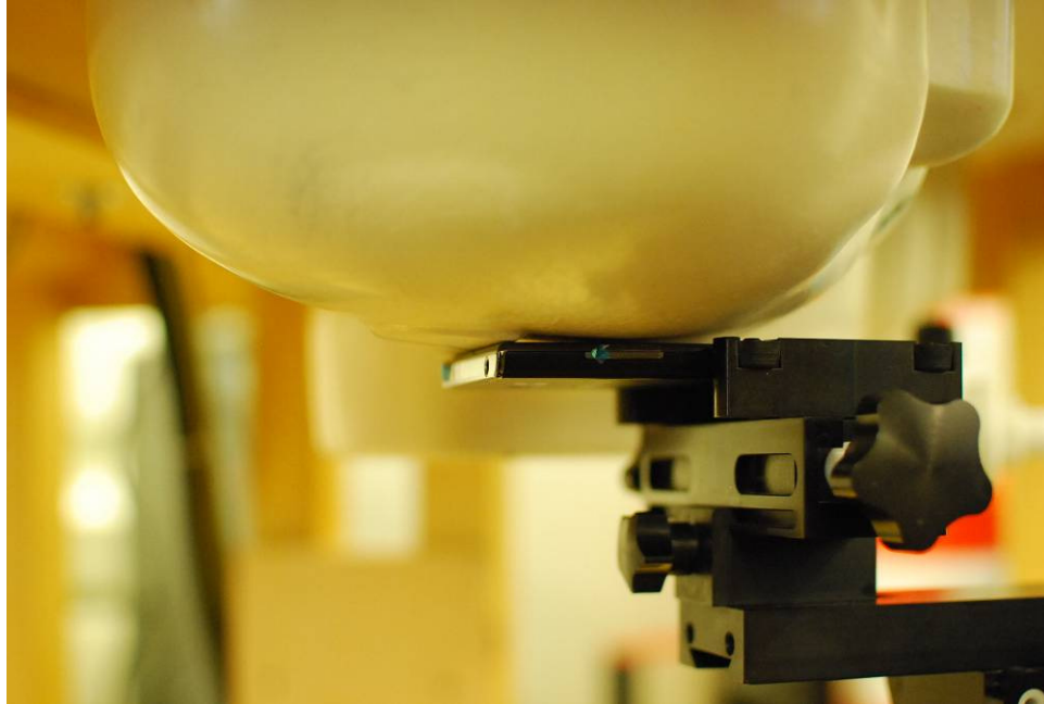
SAR Test Setup Photo 1 – Right Touch
