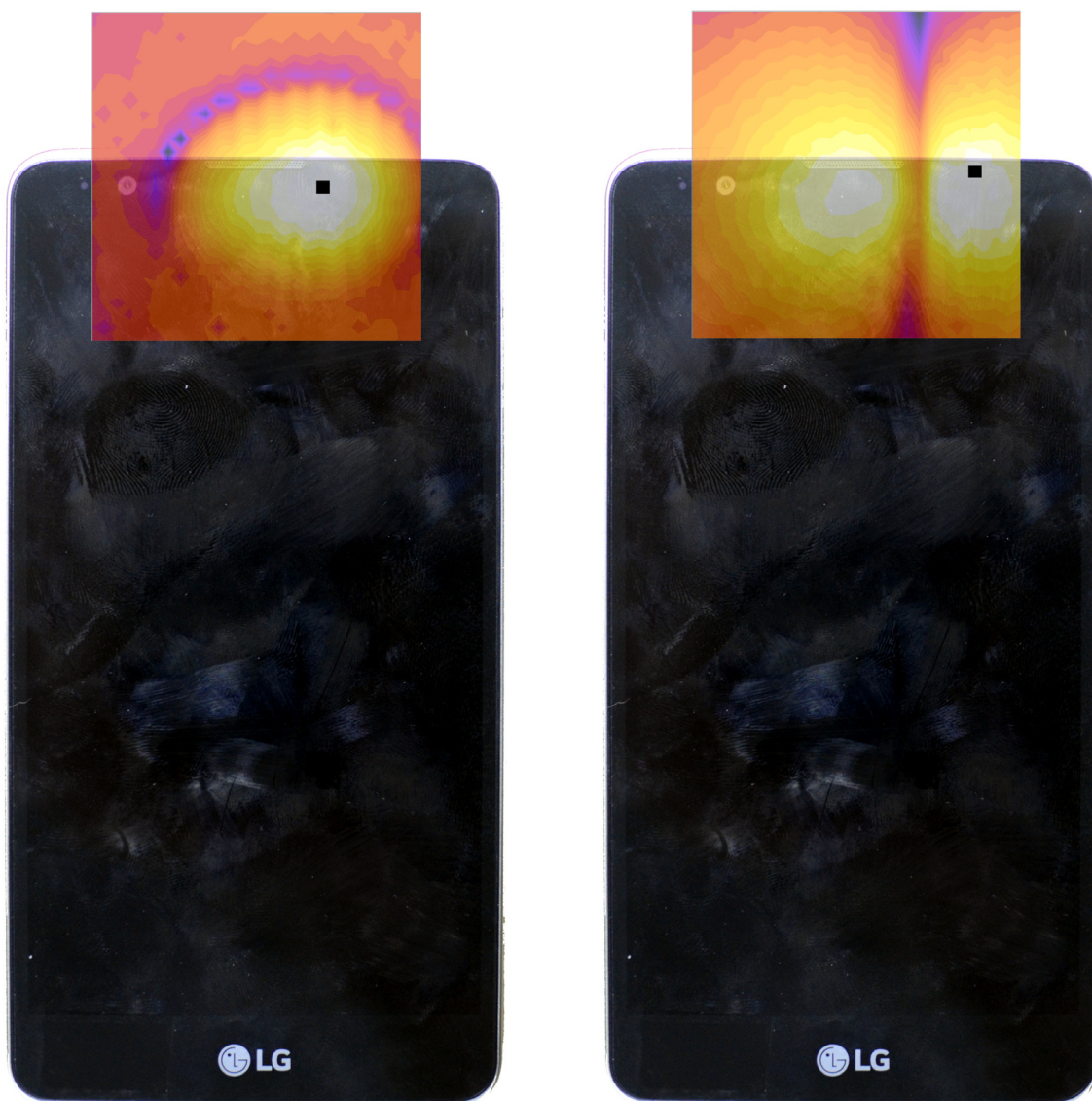
Figure 14-3 T-Coil Scan Overlay Magnetic Field Distributions
