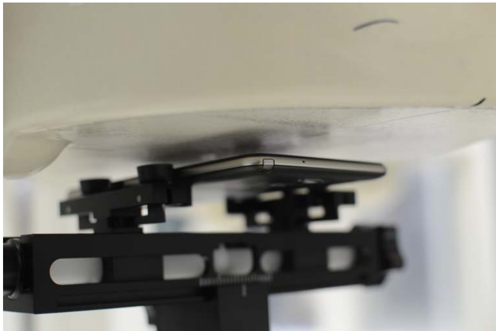
SAR Test Setup Photo 6: Front at 1.0 cm
