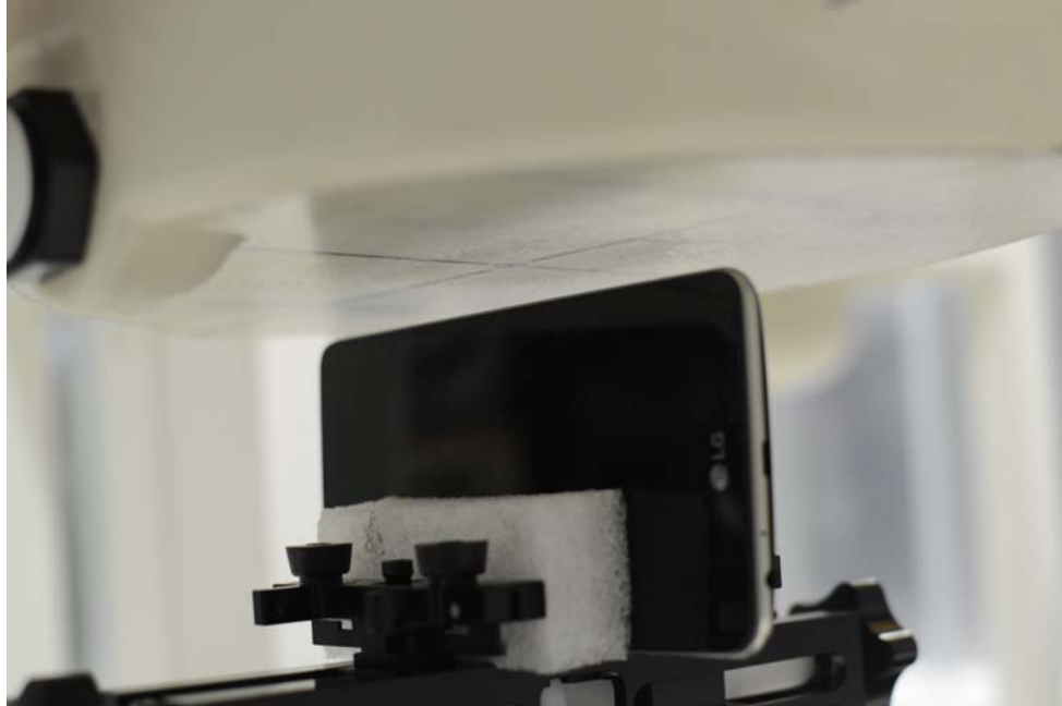
SAR Test Setup Photo 9: Right at 1.0 cm
