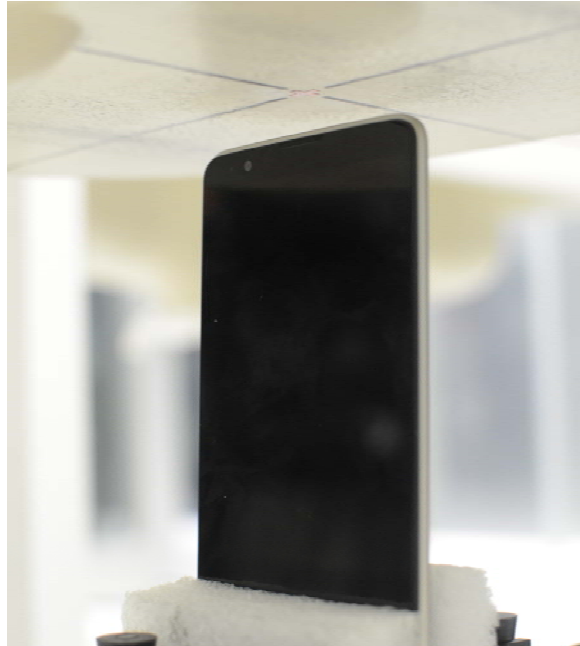
SAR Test Setup Photo 7: Top at 1.0 cm
