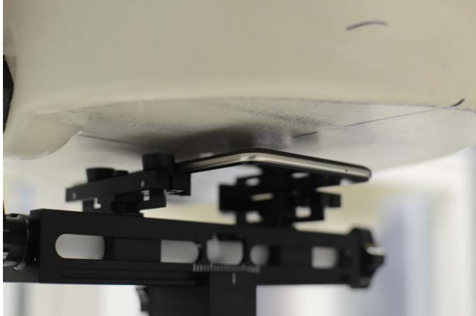
SAR Test Setup Photo 5: Back at 1.0 cm
