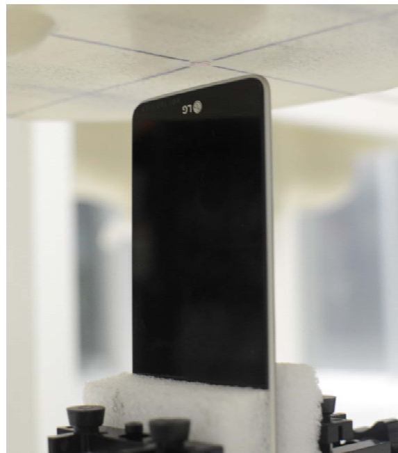
SAR Test Setup Photo 8: Bottom at 1.0 cm
