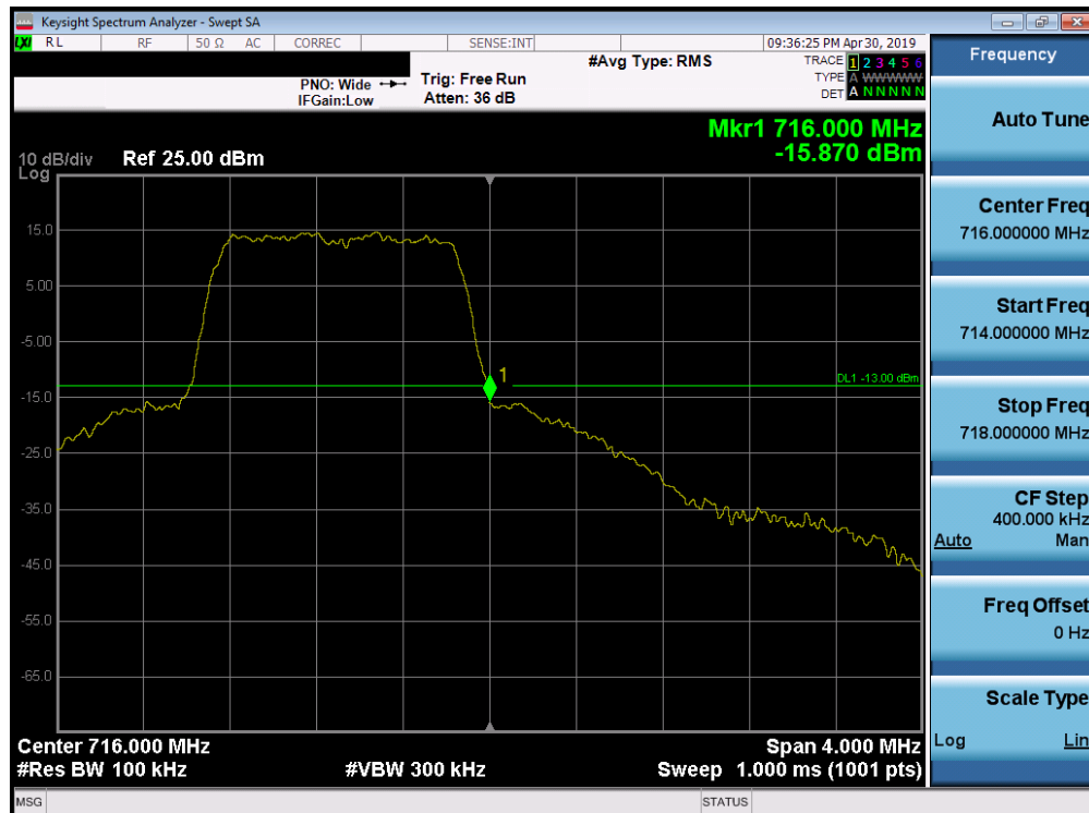
Plot 7-142. Upper Band Edge Plot (Band 12 - 1.4MHz QPSK - Full RB Configuration)
