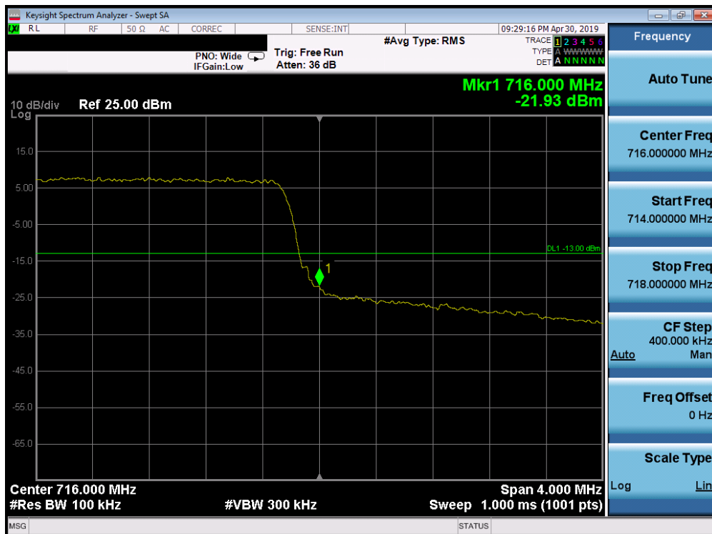
Plot 7-146. Upper Band Edge Plot (Band 12 - 5.0MHz QPSK - Full RB Configuration)
