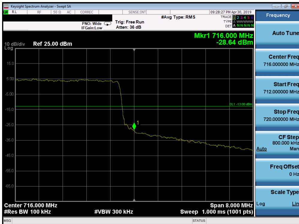
Plot 7-148. Upper Band Edge Plot (Band 12 - 10.0MHz QPSK - Full RB Configuration)
