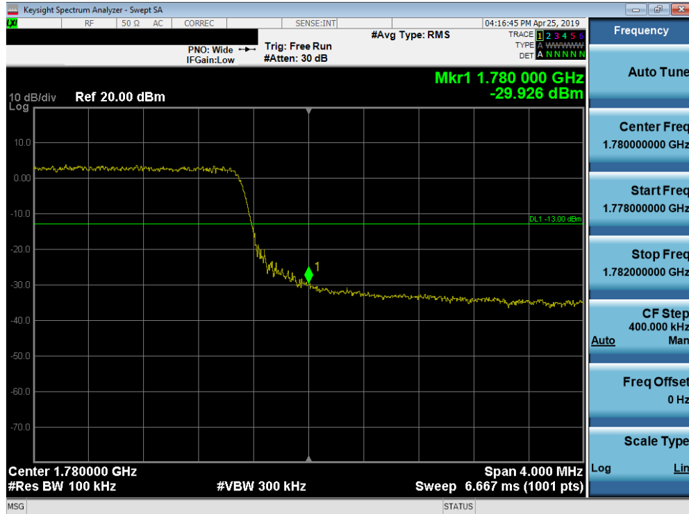
Plot 7-187. Upper Band Edge Plot (Band 66 - 10.0MHz QPSK - Full RB Configuration)
