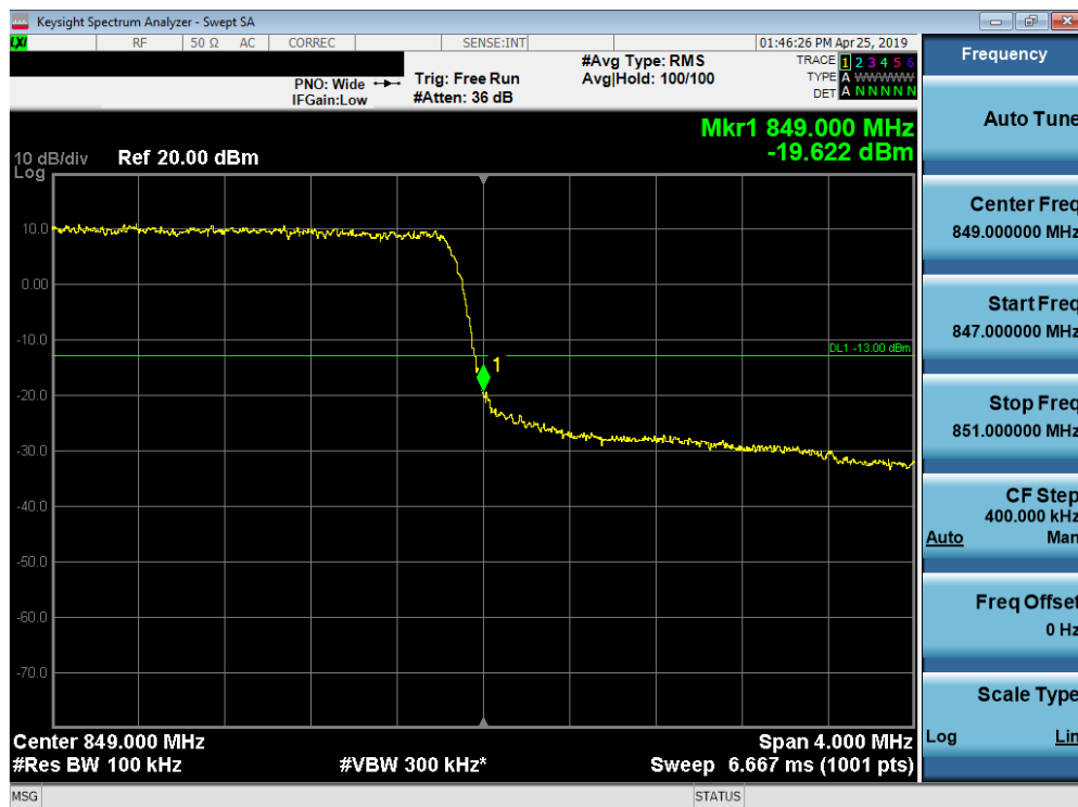
Plot 7-160. Upper Band Edge Plot (Band 5 - 3.0MHz QPSK - Full RB Configuration)
