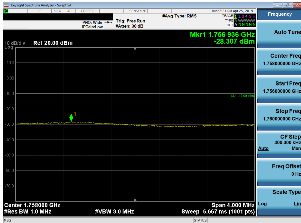
Plot 7-192. Upper Extended Band Edge Plot (Band 4 - 15.0MHz QPSK - Full RB Configuration)
