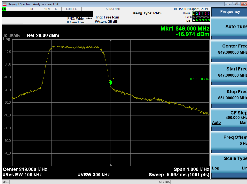
Plot 7-158. Upper Band Edge Plot (Band 5 - 1.4MHz QPSK - Full RB Configuration)
