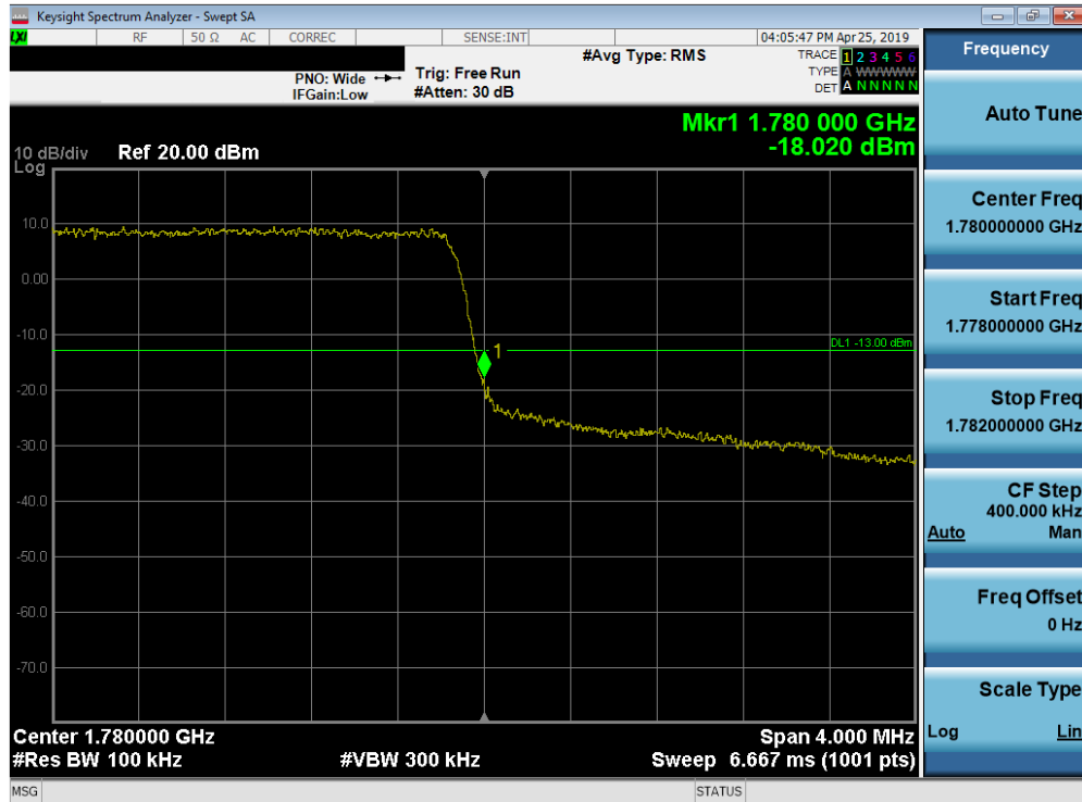
Plot 7-175. Upper Band Edge Plot (Band 66 - 3.0MHz QPSK - Full RB Configuration)
