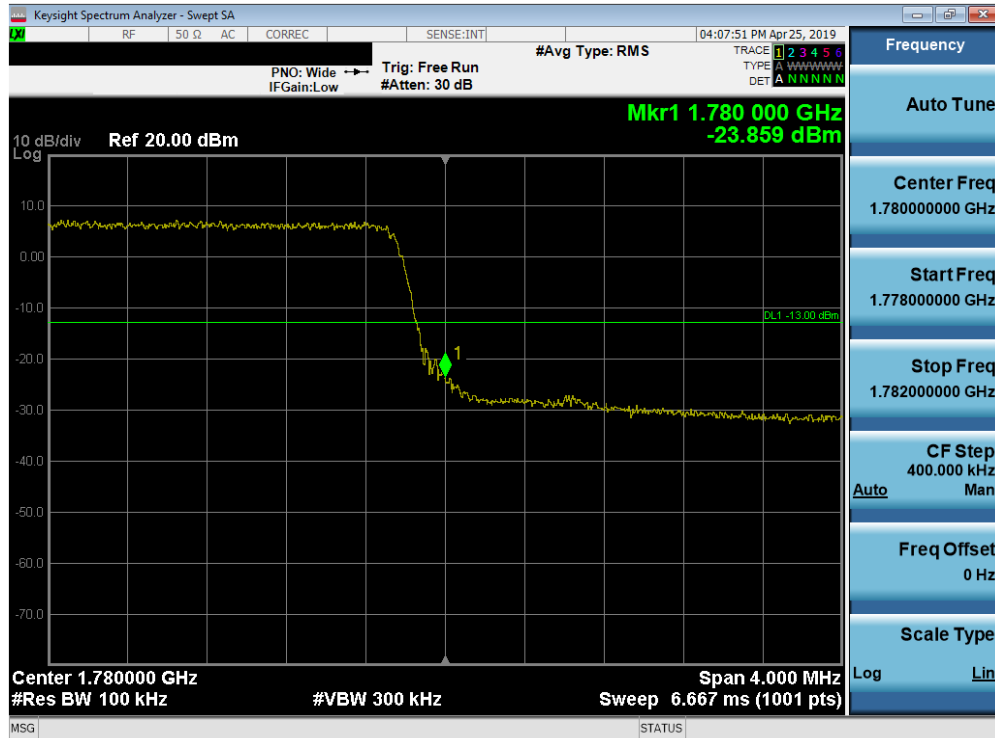
Plot 7-181. Upper Band Edge Plot (Band 66 - 5.0MHz QPSK - Full RB Configuration)
