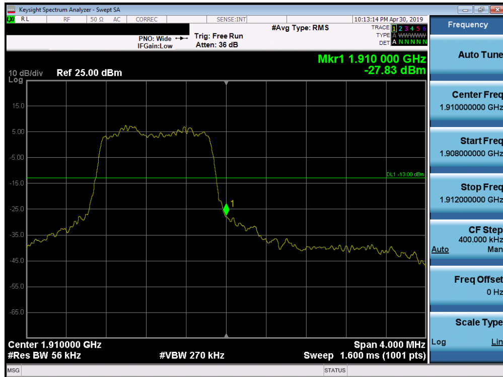
Plot 7-203. Upper Band Edge Plot (Band 2 - 1.4MHz QPSK - Full RB Configuration)
