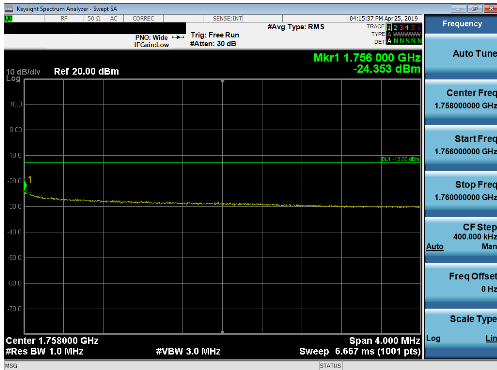
Plot 7-186. Upper Extended Band Edge Plot (Band 4 - 10.0MHz QPSK - Full RB Configuration)
