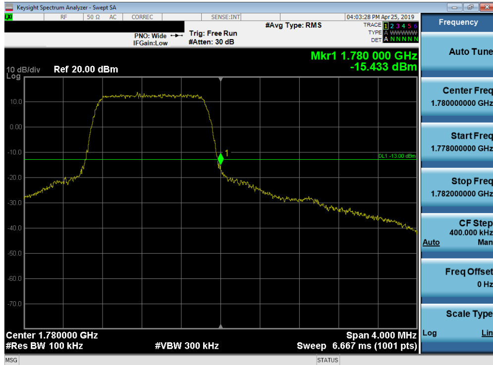
Plot 7-169. Upper Band Edge Plot (Band 66 - 1.4MHz QPSK - Full RB Configuration)
