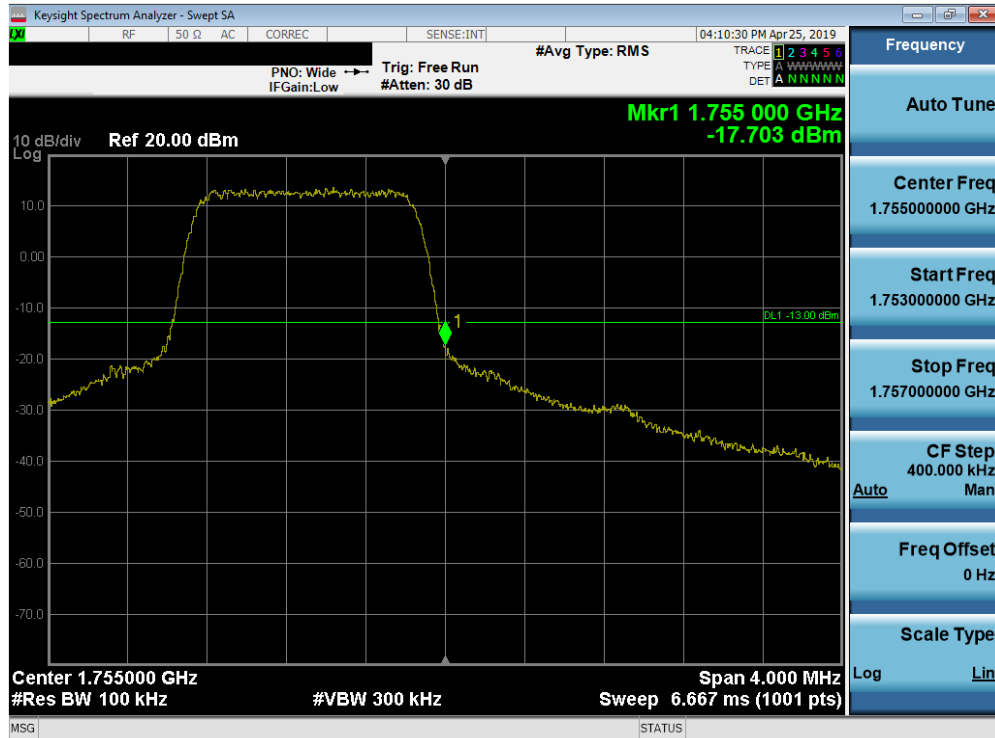
Plot 7-173. Upper Band Edge Plot (Band 4 - 3.0MHz QPSK - Full RB Configuration)
