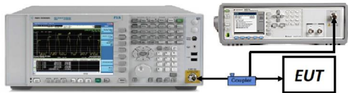
Figure 7-4. Test Instrument & Measurement Setup
