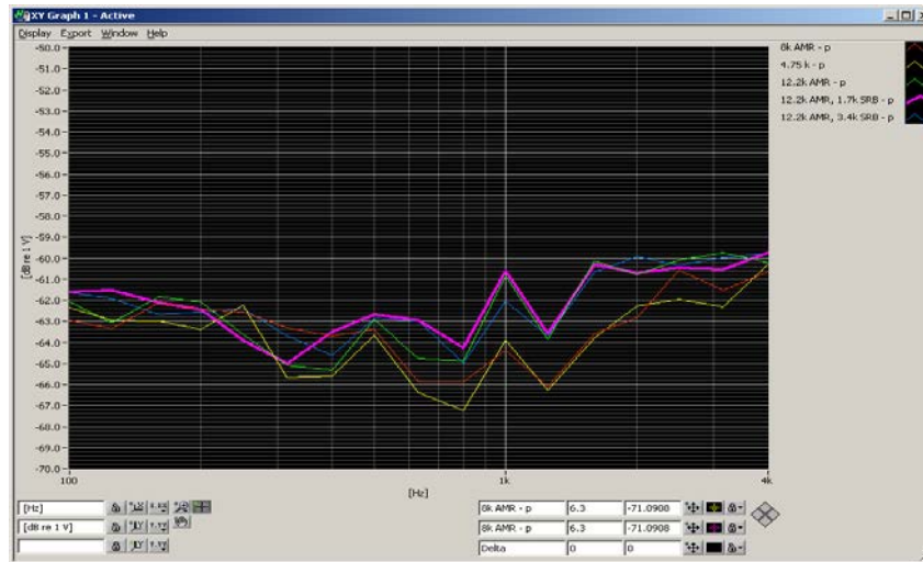
Figure 8-3 UMTS Audio Band Magnetic Noise
