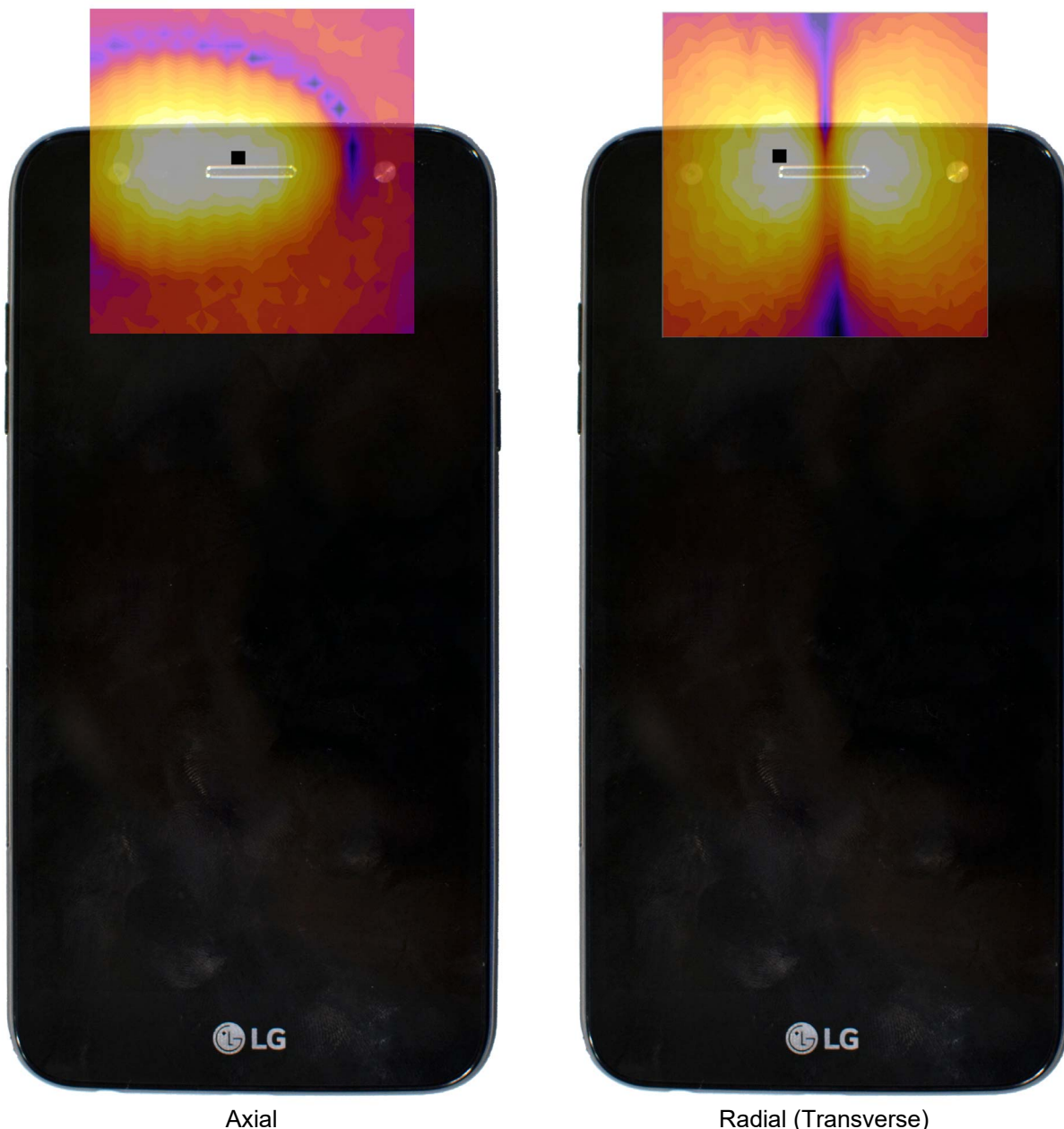
Figure 13-3 T-Coil Scan Overlay Magnetic Field Distributions
