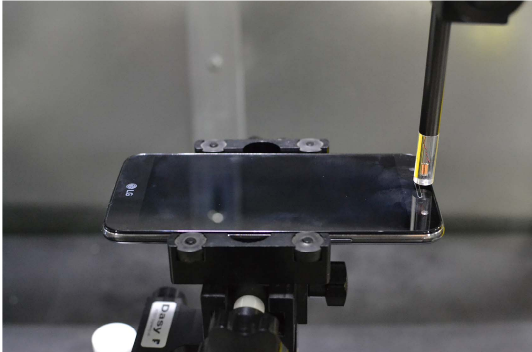
Figure 13-1 Test Setup for Wireless Device
