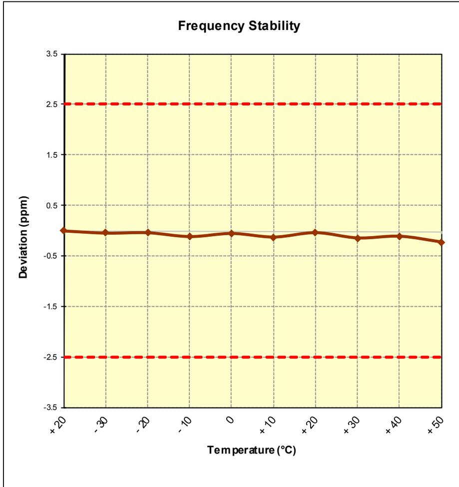
**Figure 7-8. Frequency Stability Graph (Cellular CDMA Mode – Ch. 384)**
