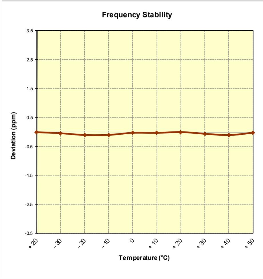
**Figure 7-9. Frequency Stability Graph (PCS CDMA Mode – Ch. 600)**
