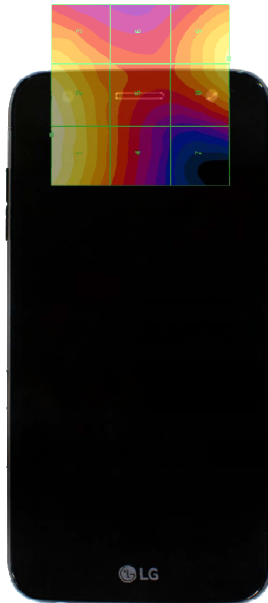
Figure 17-4 E-Field WD Scan overlay
