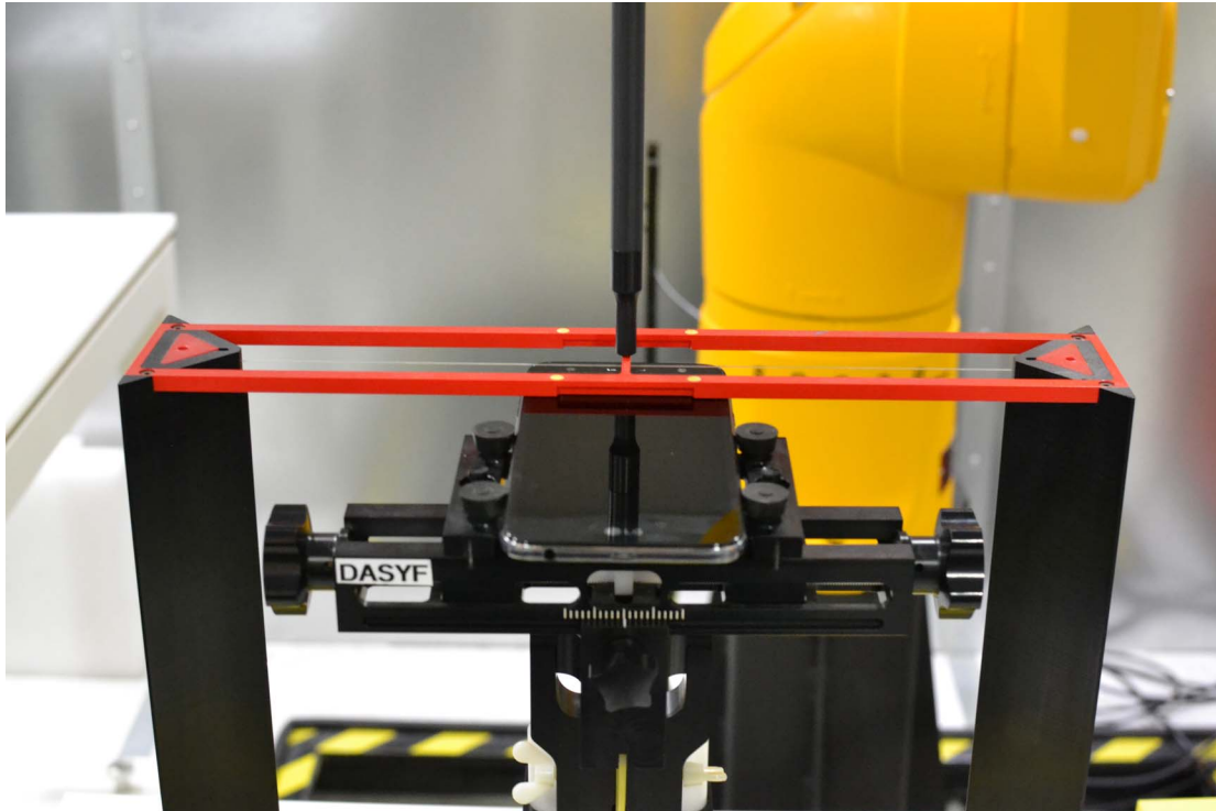
Figure 17-1 Ear Reference Point HAC Phantom Alignment
