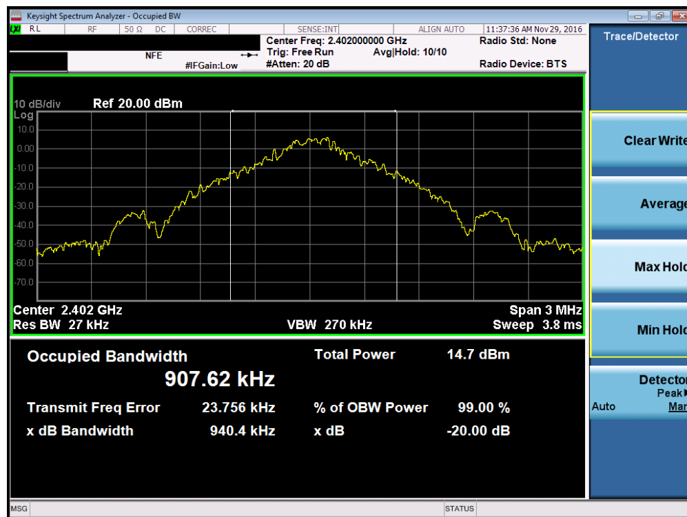
Plot 7-1. 20dB Bandwidth Plot (Bluetooth, 1Mbps – Ch. 0)
