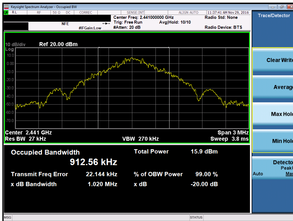
Plot 7-2. 20dB Bandwidth Plot (Bluetooth, 1Mbps – Ch. 39)
