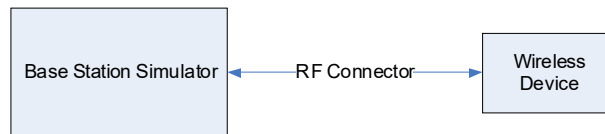
Figure 9-2 Power Measurement Setup
