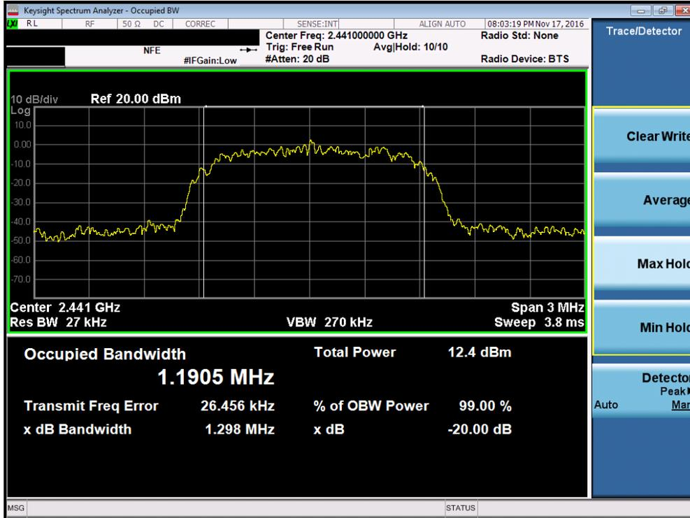
Plot 7-8. 20dB Bandwidth Plot (Bluetooth, 3Mbps – Ch. 39)
