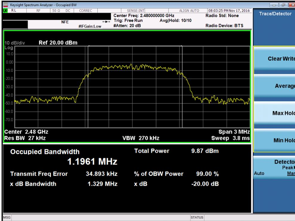
Plot 7-9. 20dB Bandwidth Plot (Bluetooth, 3Mbps – Ch. 78)
