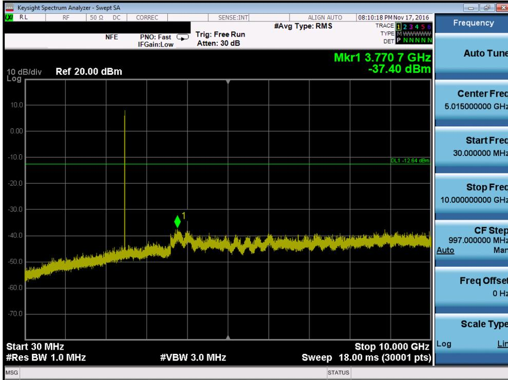
Plot 7-40. Conducted Spurious Plot (Bluetooth, 3Mbps – Ch. 78)
