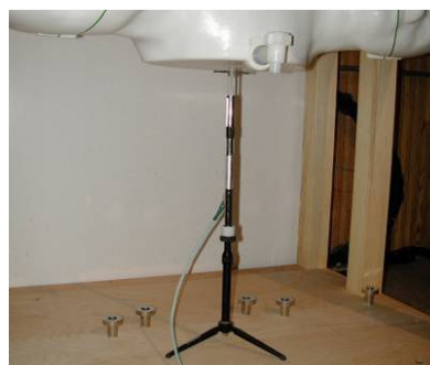
Figure 10-2 System Verification Setup Photo
