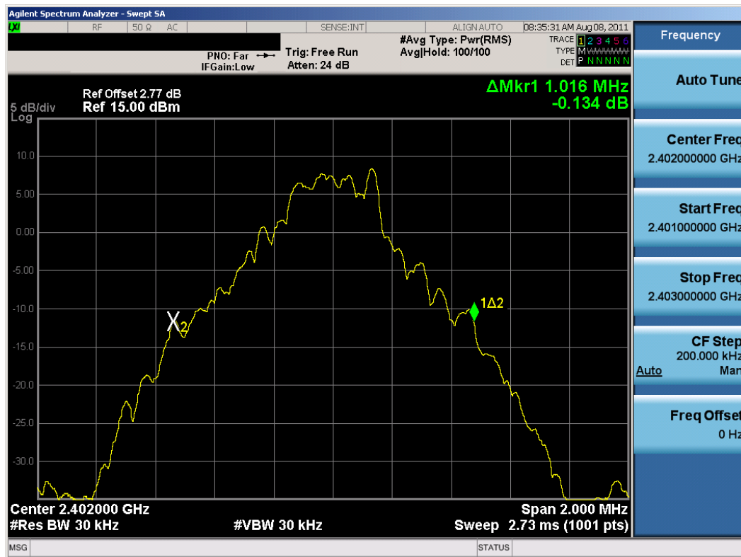
Plot 6-1. 20dB Bandwidth Plot (Bluetooth, 1Mbps - Ch. 0)
