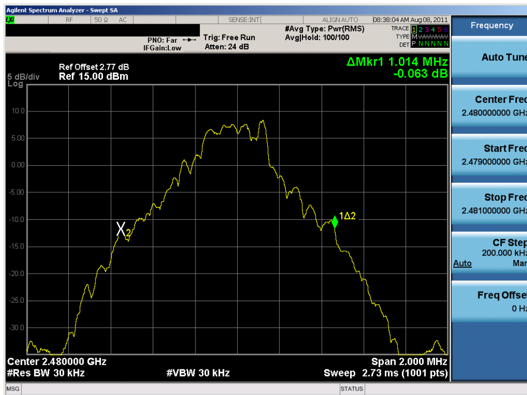
Plot 6-3. 20dB Bandwidth Plot (Bluetooth, 1Mbps – Ch. 78)
