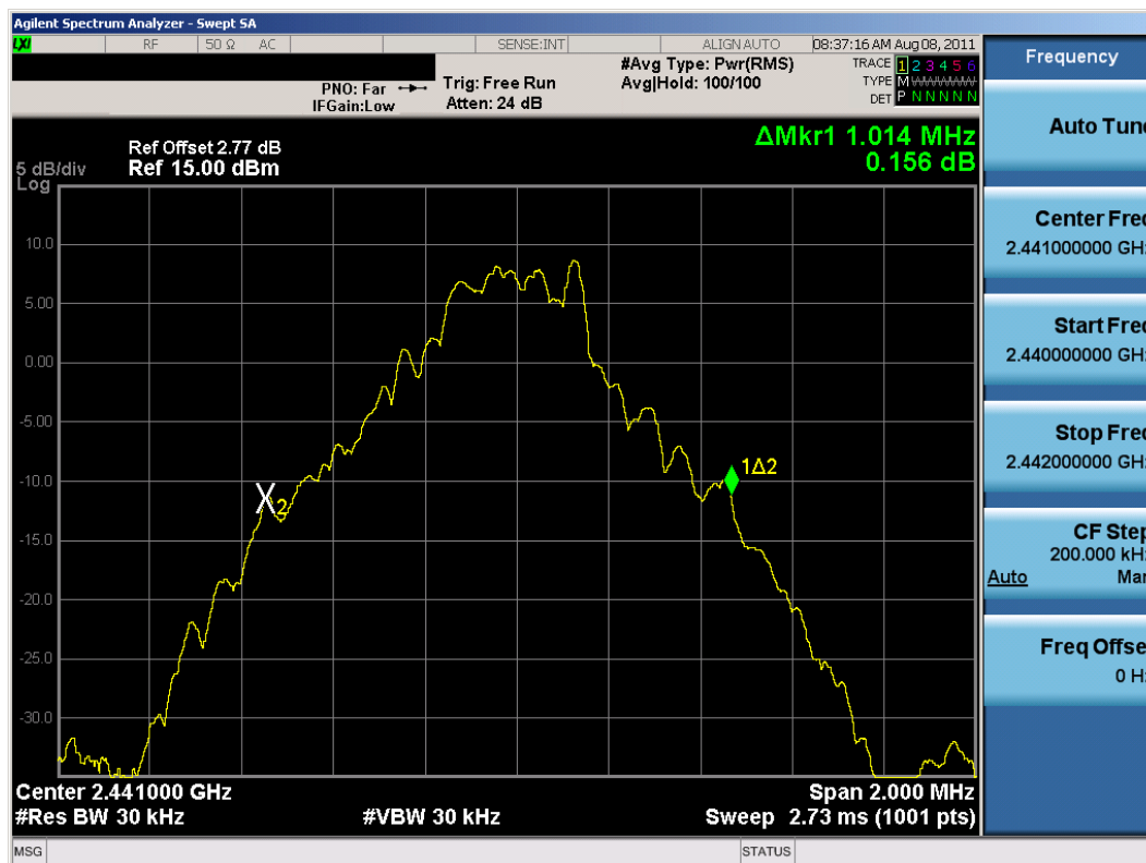
Plot 6-2. 20dB Bandwidth Plot (Bluetooth, 1Mbps - Ch. 39)
